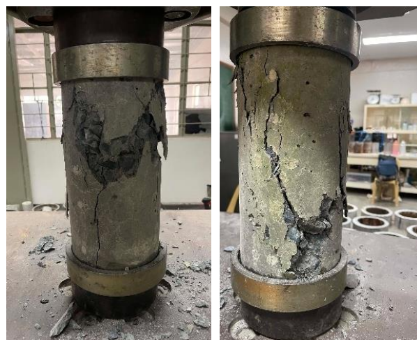
Figure 6. Sample images of fractured cylindrical samples after compressive strength tests
