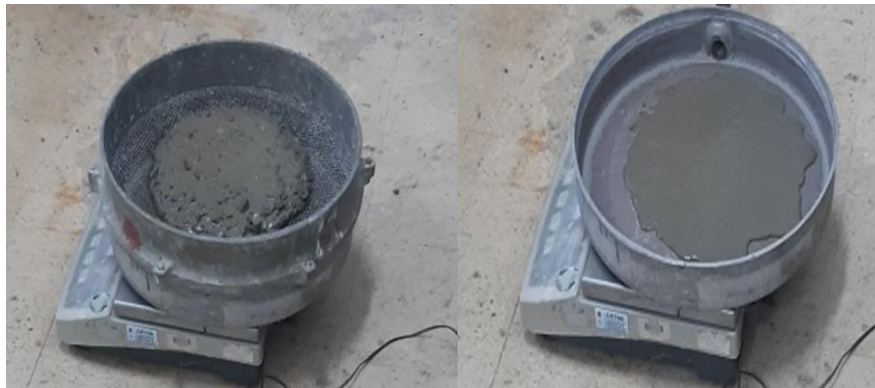
Figure 11. Sieve stability test
