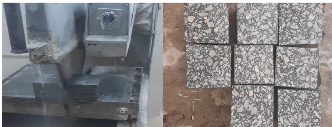
Figure 19. Cross-sectional view of sawn SCC prismatic specimens (100 × 100 mm face)
