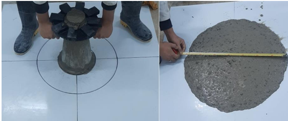
Figure 7. Abrams cone spread test
