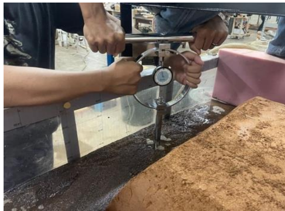
Figure 8. Hand Cone Penetrometer (HCP) Testing
