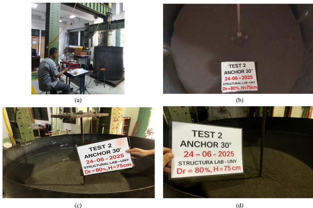
Figure 6. (a) Pullout testing of the jack anchor (b) Backfilling over the jack-like ground anchor; (c) Jack anchor ready for testing; (d) Jack anchor after testing
