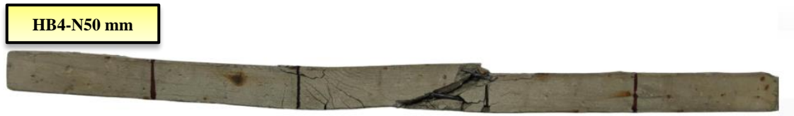
Figure 25. Cracking propagation of Normal stirrups for HB1, HB2, HB3, and HB4
