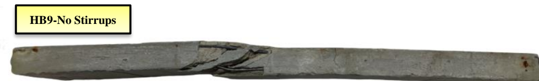
Figure 27. Cracking propagation for specimen HB9, which has no stirrups
