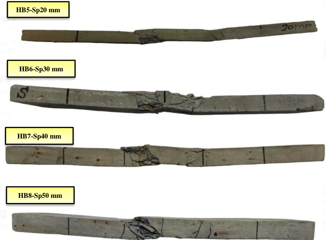
Figure 26. Cracking propagation of staggered spiral for HB5, HB6, HB7, and HB8
