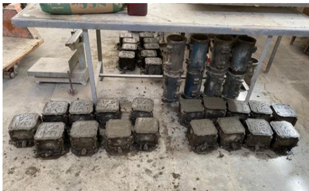
(a) Samples for Compressive and Tensile Strengths
