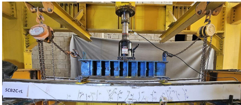
Figure 22. Tested specimen SCB2C-rL and Failure Mode Flexure
