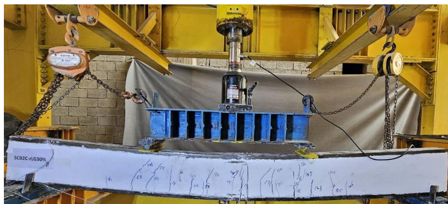
Figure 25. Tested specimen SCB2C-rLG30% and Failure Mode
