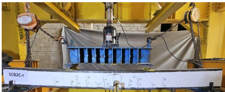
Figure 21. Tested specimen SCB2C-r and Failure Mode Flexure
