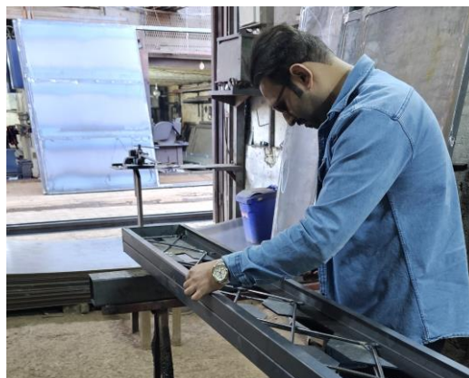
Figure 4. Lacing reinforcement by welding
