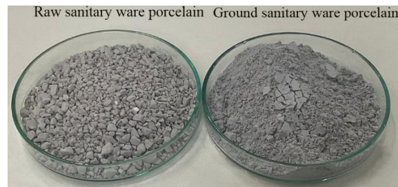
Figure 2. Raw material before and after ground porcelain material
