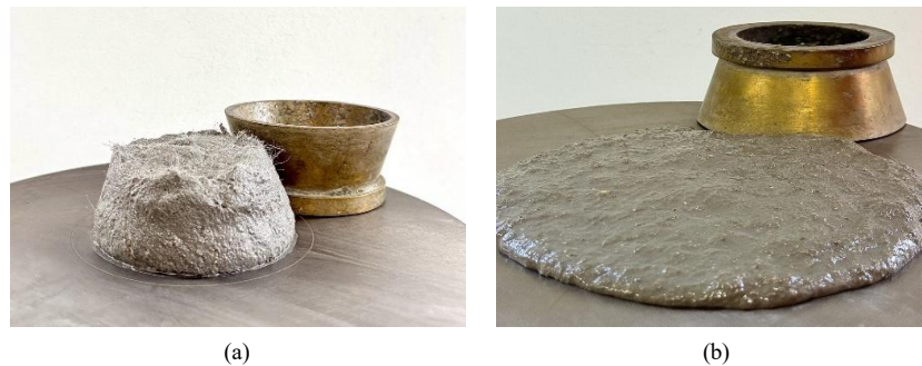
Figure 5. Workability of Porcelain based geopolymer with PP fiber mortar (a) Mini-slump (b) Flow-table
