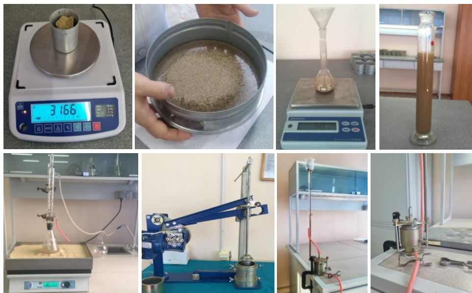
Figure 1. Preparing Fragments of the process of studying the characteristics of fine-earth samples: the duration of water filtration, the level of water reduction during filtration, the filtration coefficient, mass, humidity, density before and after testing.
