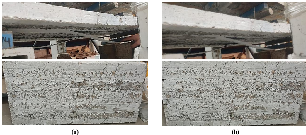
Figure 7. Mode failure and crack pattern (a) S1-S and (b) S2-S
