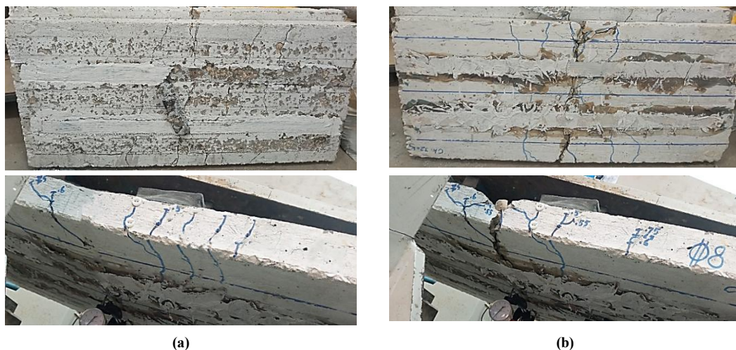
Figure 8. Mode failure and crack pattern (a) S1-C and (b) S2-C
