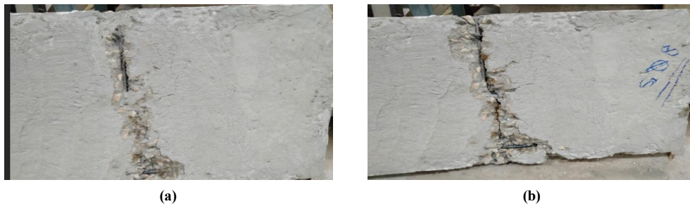
Figure 6. Mode failure and crack pattern (a) S1 and (b) S2
