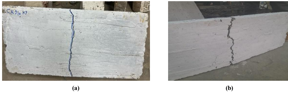
Figure 9. Mode failure and crack pattern (a) S1-E and (b) S2-E
