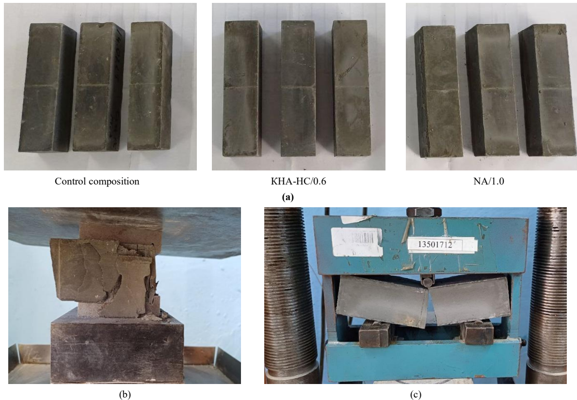
Figure 7. Experimental HPC samples: (a) appearance; (b) in the compressive strength test; (c) in the flexural strength test
