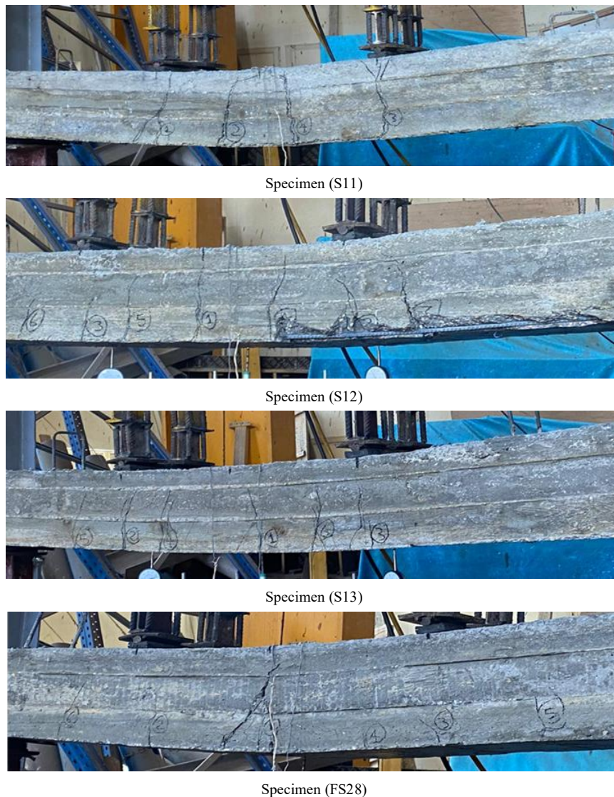
Figure 12. Crack pattern of full-thickness slab group (E)
