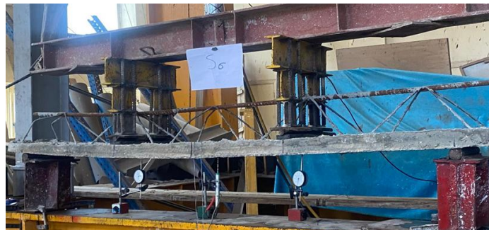
Figure 9. Stirrups Welding Failure in Semi-Precast Slab with 22 mm bar diameter
