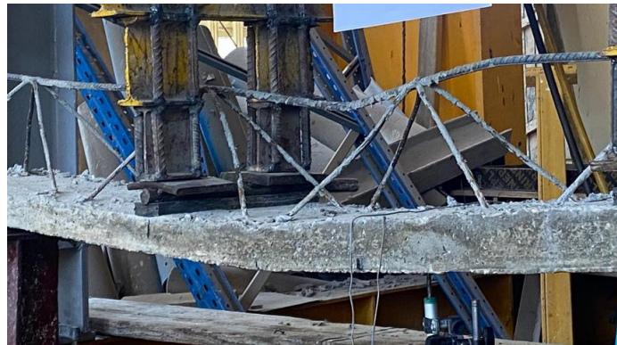
Figure 8. Top-Chord Bar Buckling in Semi-Precast Slab with 12 mm bar diameter
