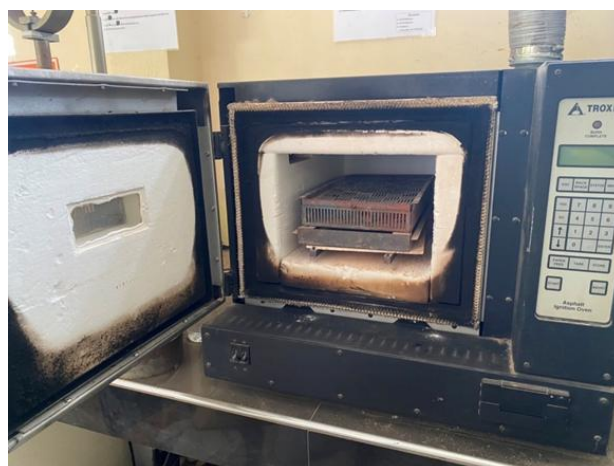
Figure 7. Determination of asphalt content
