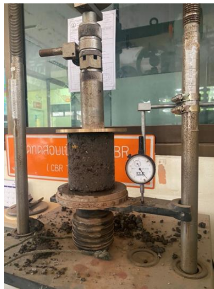
Figure 6. Unconfined compressive strength (UCS) test
