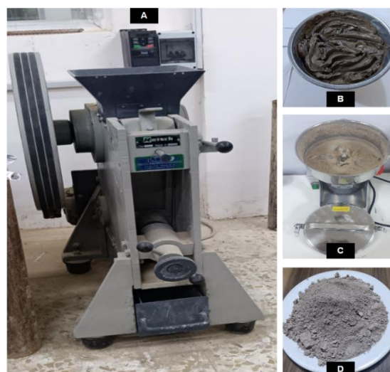
Figure 2. Sequential Stages of Soil Sample Preparation (A) Jaw crusher, (B) Raw clay, (C) Grinder and mixer, (D) Powdered soil
