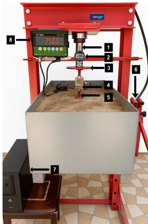
Figure 4. Model Footing Test Apparatus with Labeled Components (1- Hydraulic Press, 2- Dial Gauge, 3- Loading Plate Connection, 4- Load Cell, 5- Model Footing, 6- Manual Jack Handle, 7- Uninterruptible Power Supply, 8- Load indicator)
