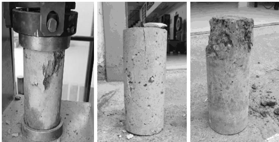
Figure 4. Compression test failure patterns of the concrete samples
