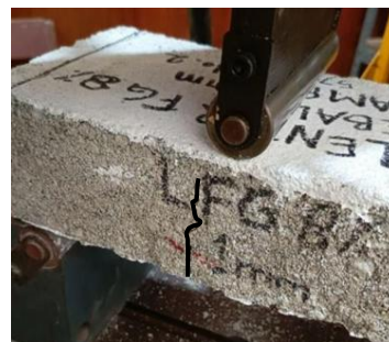
(b) The sample of 1 mm thick fiberglass painted Concrete Block cracked in the middle.
