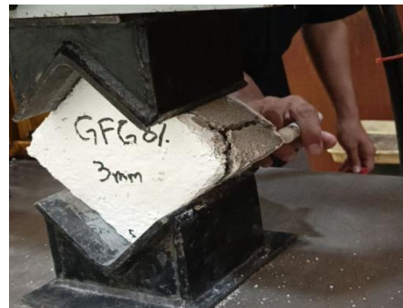
(d) Concrete Block with 3 mm-thick fiberglass paint can be seen in the image. There were no cracks in the paint layer, but there were cracks on the inside of the block, and the paint can be seen to have only shrunk.
