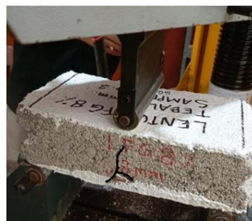
(d) A sample of 3 mm thick fiberglass painted Concrete Block appears to have cracks in the middle.
