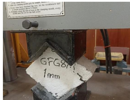
(b) Concrete Block with 1mm thick fiberglass paint experienced cracks on the right side and shrinkage of the paint on the left side.
