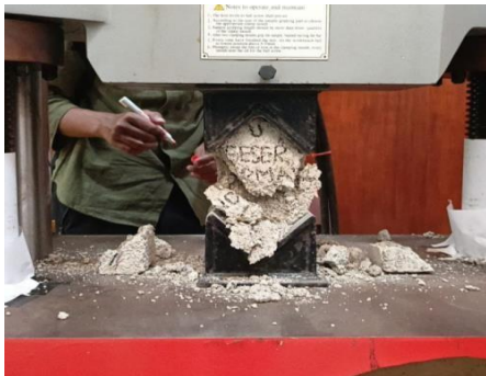
(a) The control shear sample is seen in the image to have collapsed when given a load.
