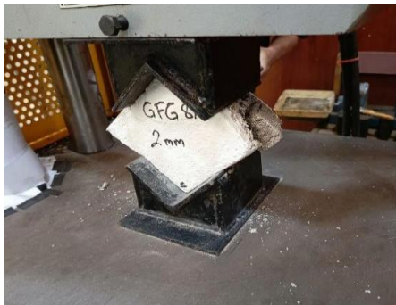
(c) The concrete block with 2 mm thick fiberglass paint did not experience cracks in the paint layer but experienced cracks on the inside of the block, and it was seen that the paint only experienced shrinkage.
