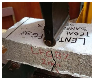
(c) The sample of 2 mm-thick fiberglass-painted Concrete Block cracked in the middle.
