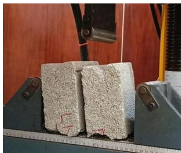
(a) The control sample can be seen as collapsed in the middle of the image.
