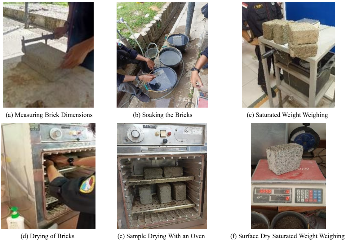
Figure 2. Concrete Block characteristics inspection process
