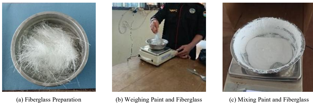
Figure 4. Fiberglass Paint Production Process
