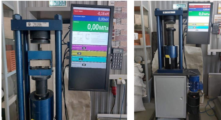
Figure 2. Determination of cement activity, Left – in flexural, right – in compression
