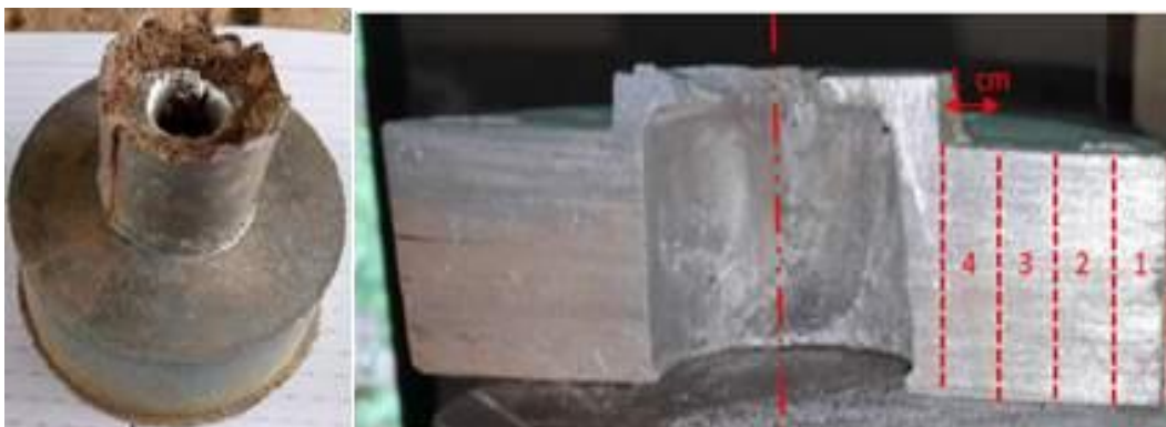
Figure 4. Results of the casting process and designation of specimen number
