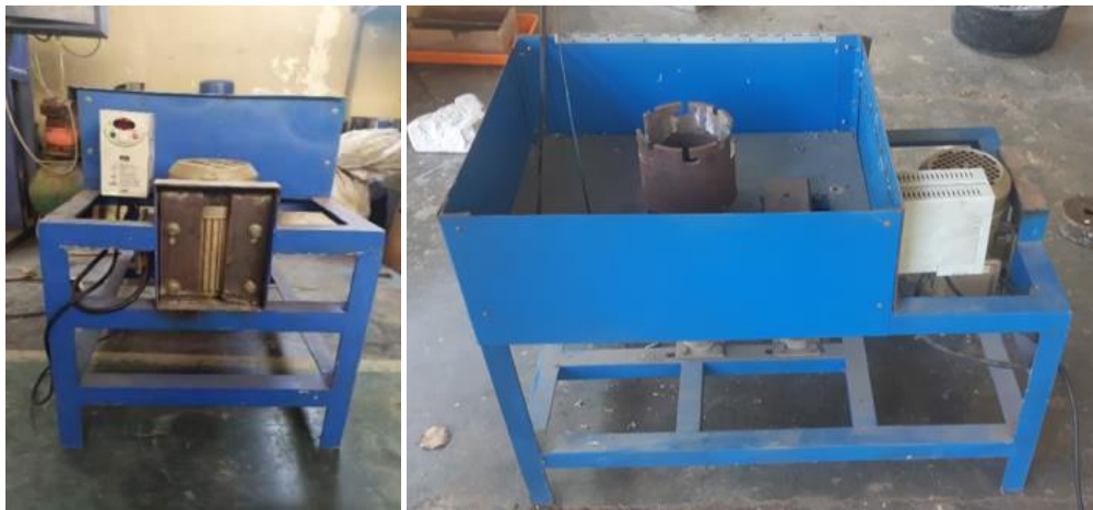
Figure 3. Vertical centrifugal casting machine
