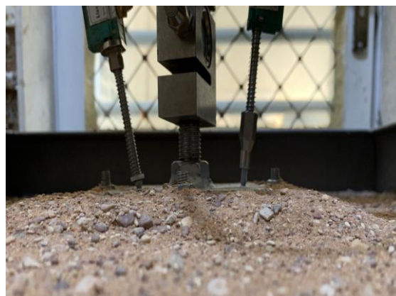
Figure 14. Failure Surface of Skirted footing at \alpha = 0^\circ
