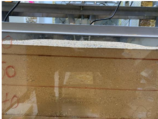
Figure 17. Failure Surface of Skirted footing at \alpha = 45^\circ
