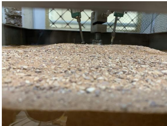
Figure 16. Failure Surface of Skirted footing at \alpha = 30^\circ
