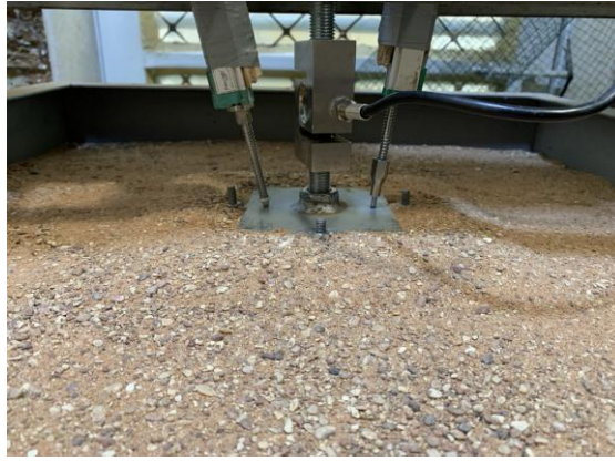
Figure 15. Failure Surface of Skirted footing at \alpha = 15^\circ
