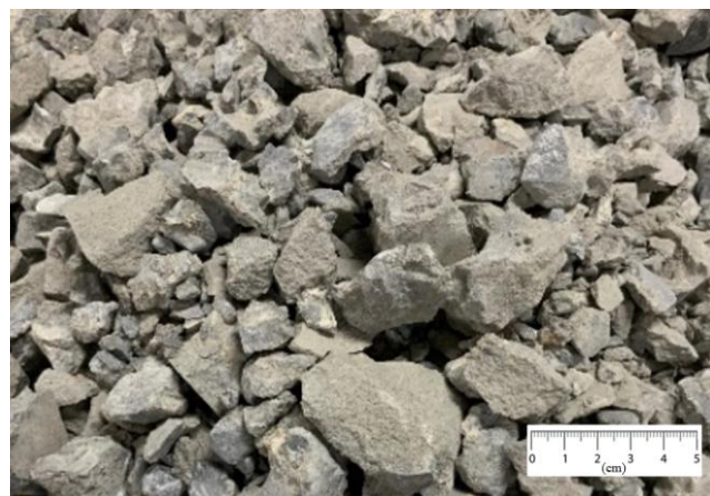
a) Recycled aggregates sourced from leftover concrete piles
