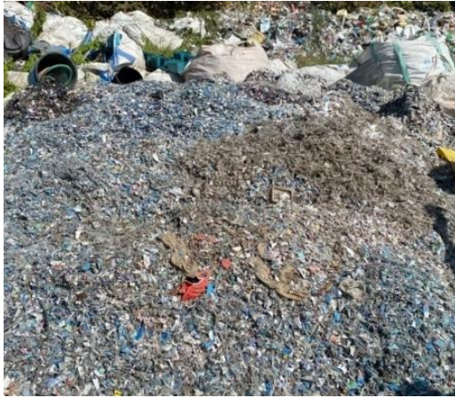
b) Plastics used as a replacement for fine aggregates
