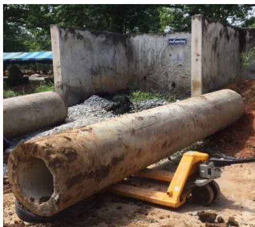
a) Recycled aggregates sourced from leftover concrete piles
