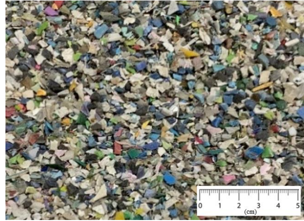
b) Plastics used as a replacement for fine aggregates
