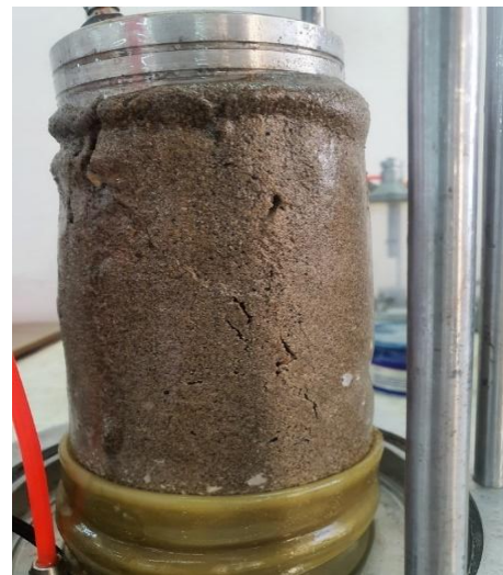
(b) Shear failure plane
