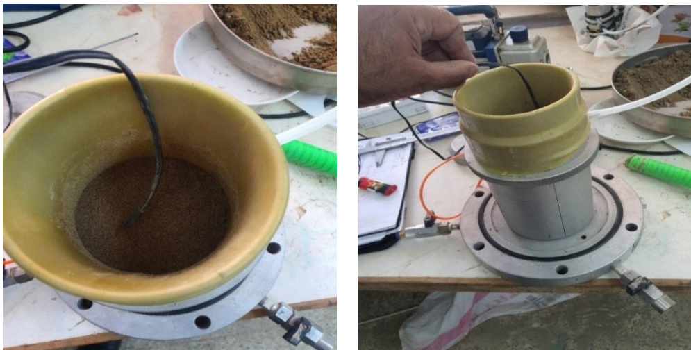
Figure 4. Remolded soil samples with the same void ratio and degree of saturation
