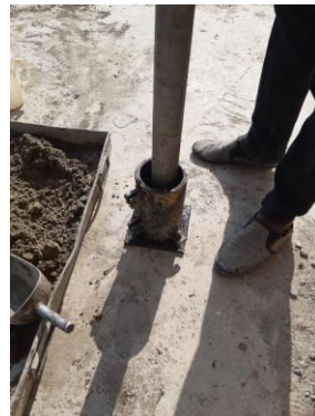
Figure 11. Pouring of wet soil-cement mix in the cylindrical mould and compaction in layers
