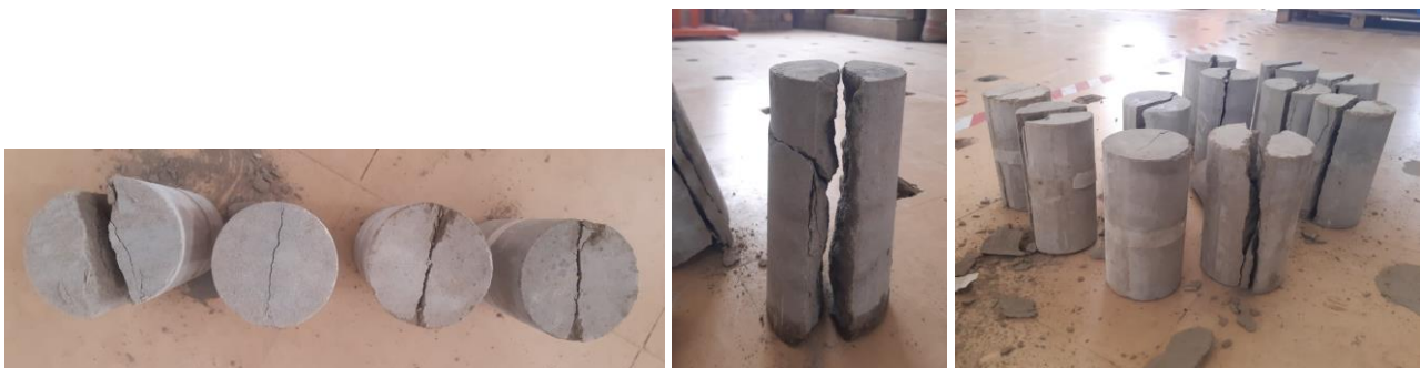
Figure 32. Failure patterns/mechanisms of cement-stabilized rammed-earth specimens after the tension failure
