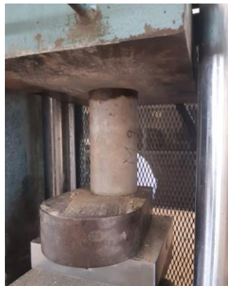
Figure 21. Cement-stabilized rammed-earth specimens under the application of compressive load
