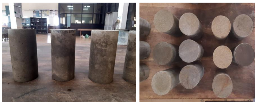
Figure 18. Cement-stabilized rammed-earth specimens after curing and ambient drying, and before testing
