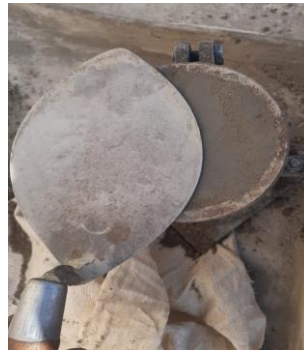
Figure 13. Finishing of the cement-stabilized rammed-earth specimen in the cylindrical mould
