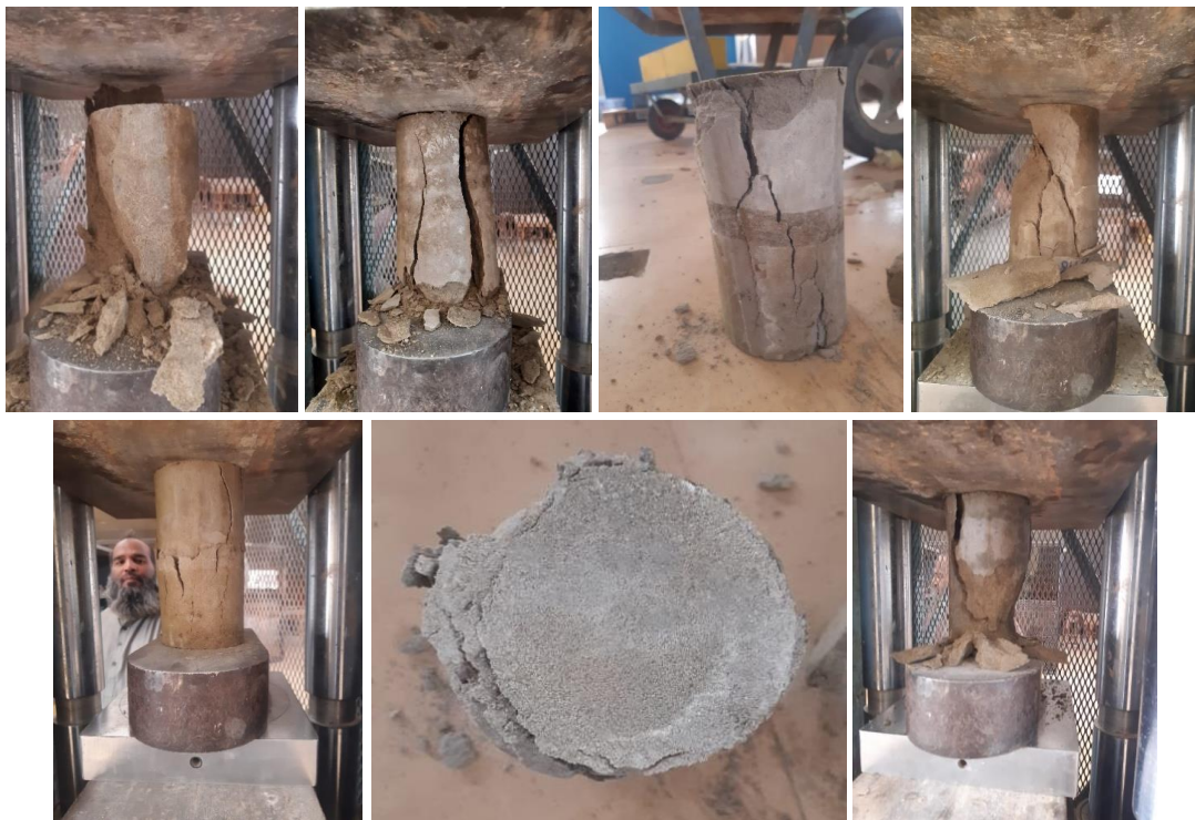
Figure 27. Failure patterns/mechanisms of cement-stabilized rammed-earth specimens after the compression failure
