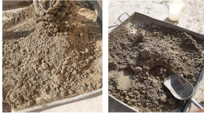
Figure 10. Wet mixing of soil-cement material
