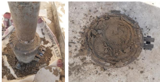
Figure 12. Compacted wet soil-cement mix in the cylindrical mould up to complete height
