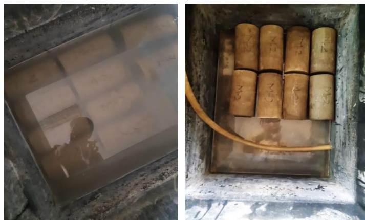
Figure 17. Curing of cement-stabilized rammed-earth specimens
