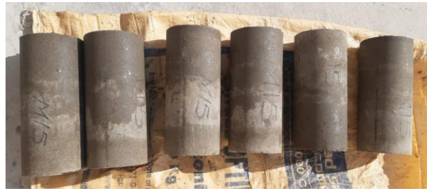
Figure 16. Labelling of cement-stabilized rammed-earth specimens
