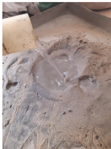
Figure 9. Pouring of water in the soil-cement mix
