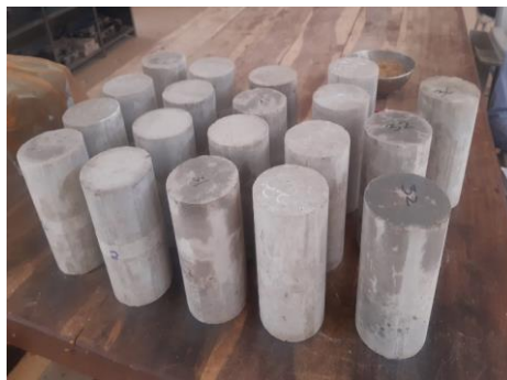
Figure 20. Cement-stabilized rammed-earth specimens before the compressive strength test
