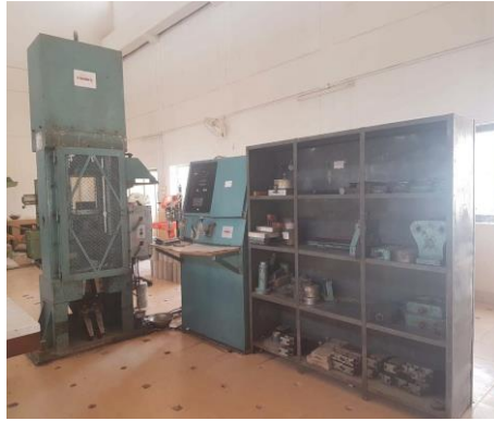
Figure 19. Universal testing machine (UTM at the Department of Civil Engineering, Mehran UET, Jamshoro
