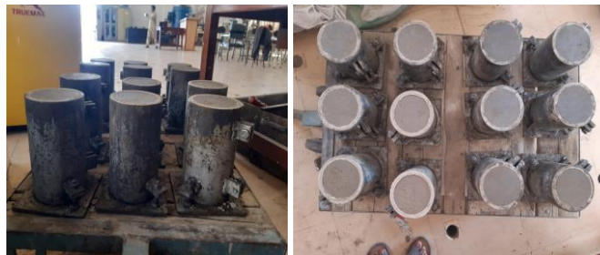
Figure 14. Cement-stabilized rammed-earth specimens cast in the cylindrical moulds
