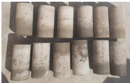
Figure 15. Demoulded cement-stabilized rammed-earth specimens
