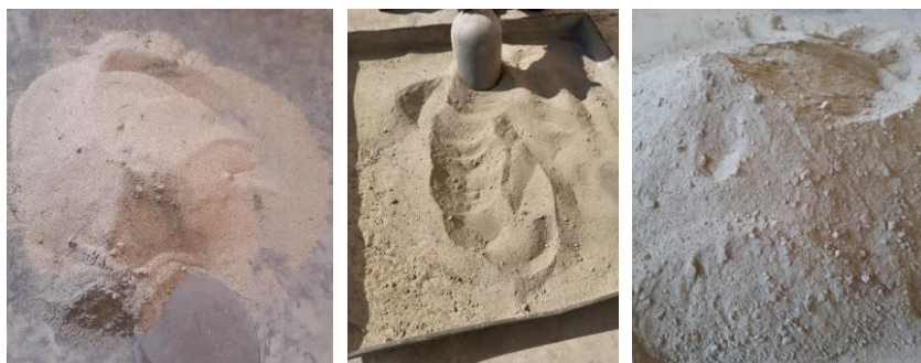
Figure 7. Dry hand blending of clay and Thar Desert sand
