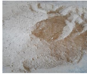
Figure 8. Dry blending of cement with sand-clay mix
