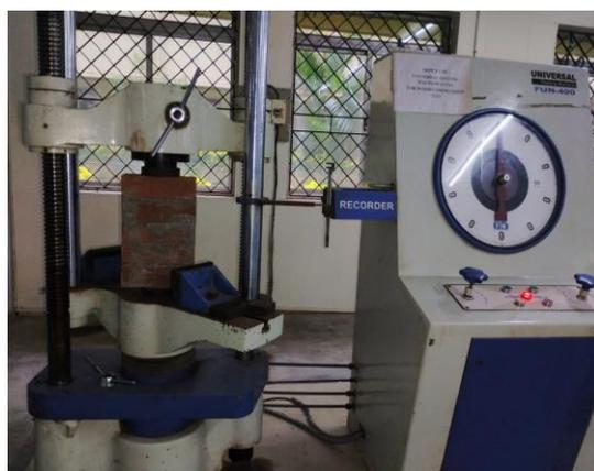
**Figure 13. UTM for Prism Test**
