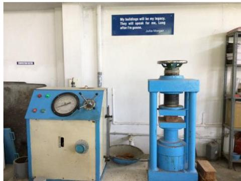
Figure 7. CTM for Compressive Strength
