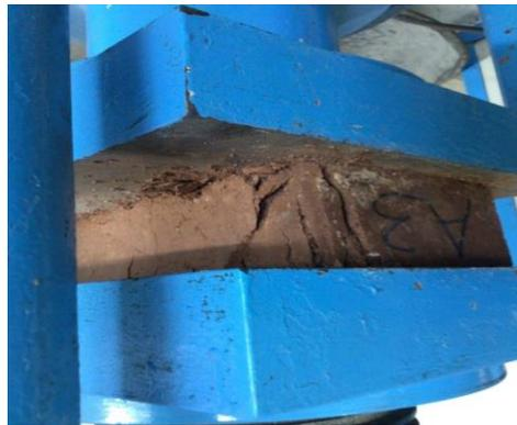
Figure 17. Crack and failure pattern for conventional block (SSB)
