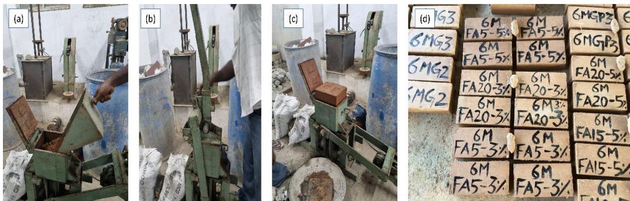
**Figure 6. Process of Making the Bricks with Different Molar of NaOH**
