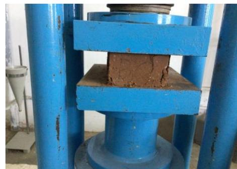
Figure 19. Crack and failure pattern for sample 7MB6
