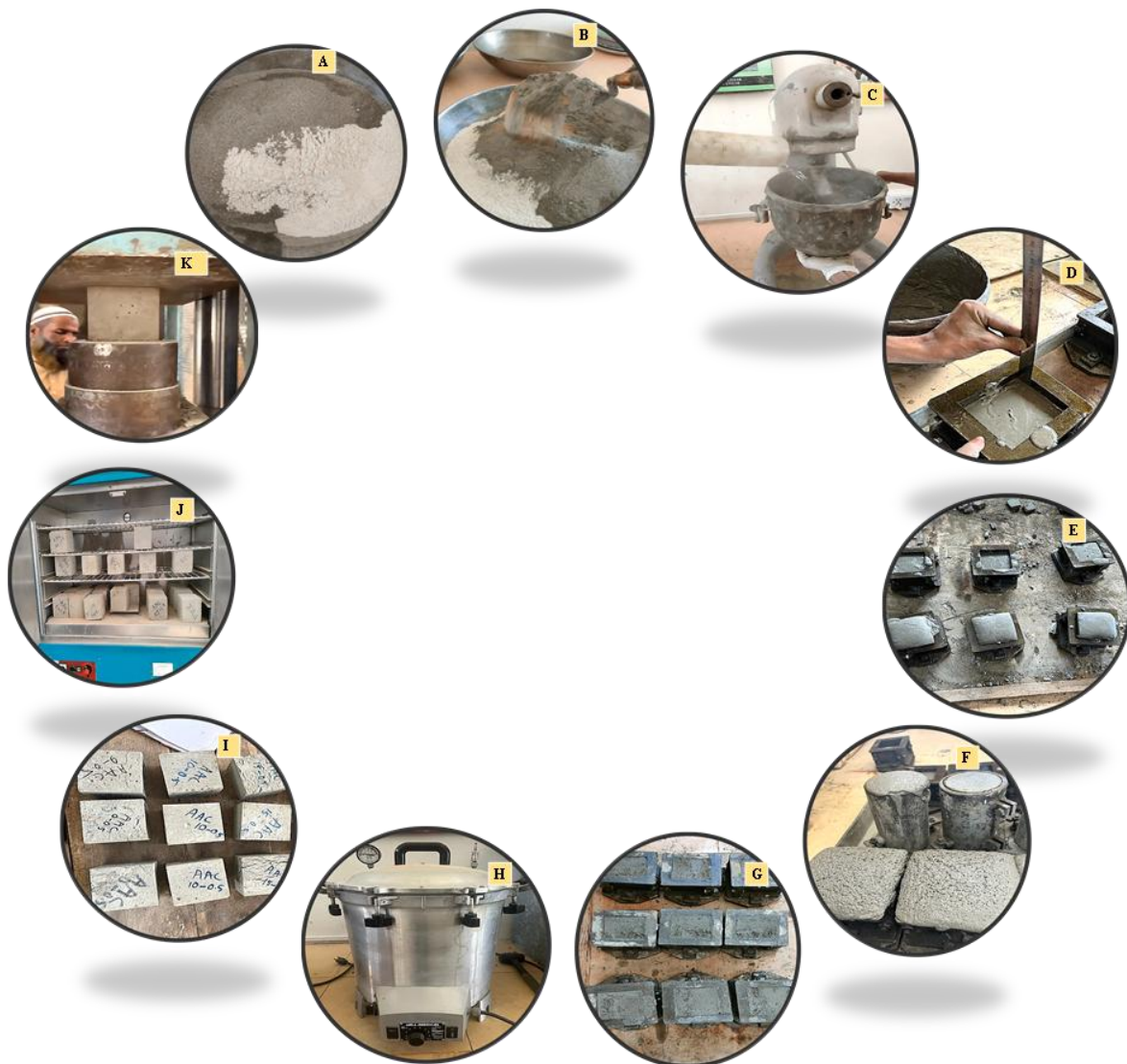
Figure 12. Experimental Procedure for Compressive Strength Testing. (A-C) Mixing of materials: Preparation of the components for specimen formation. (D) Casting of cubes: Molding the prepared mixture into standardized shapes using steel molds. (E-F) Aeration of cubes: Ensuring uniform air distribution within the cubes. (G) Cutting of cubes: Shaping the specimens to meet uniformity standards for testing. (H) Steam curing: Application of controlled steam at specified pressures (0.5, 1, and 1.5 bar) for 8 hours, and by conventional curing for 7, 14, and 28 days. (I-J) Oven drying and compressive strength testing: Samples dried at 105 \pm 5^\circ\text{C} for 24 hours as per ASTM C642. (K) Final specimen preparation: Overview of the post-curing specimen, ready for final testing and analysis.
