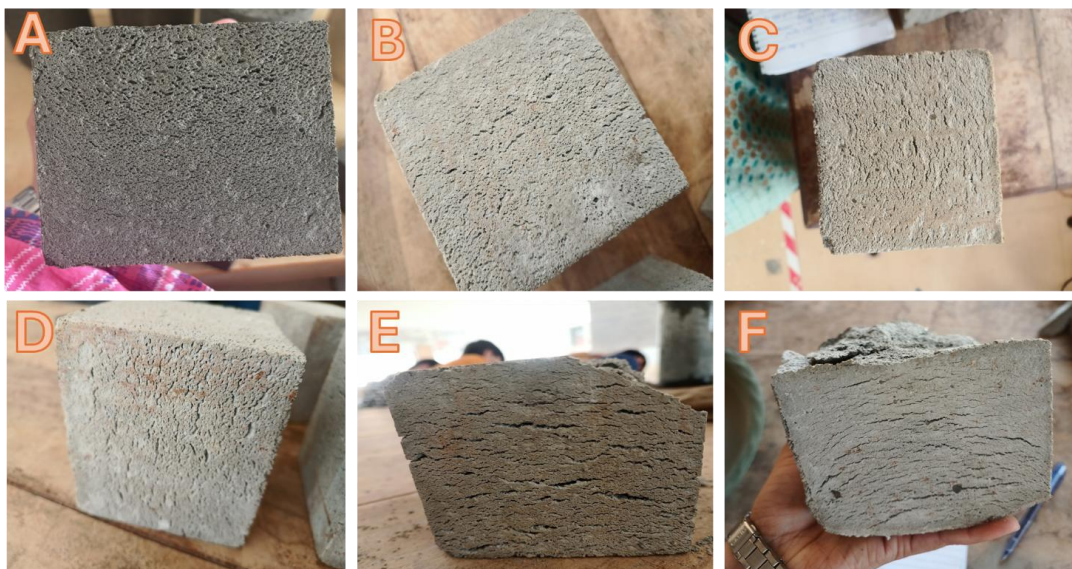
Figure 17. Crack patterns of Aerated Concrete
