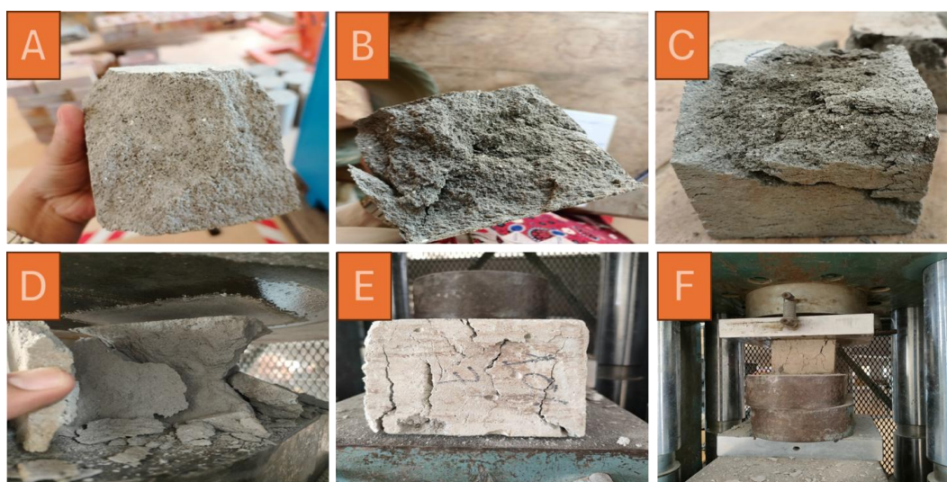
Figure 18. Failure Patterns of Aerated Concrete
