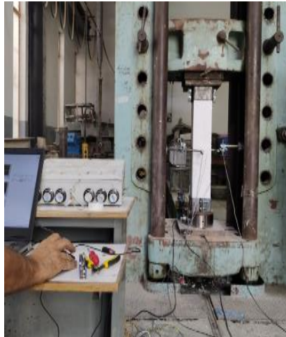
Figure 2. Testing the apparatus and instrumentation for concrete-encased CFST column
