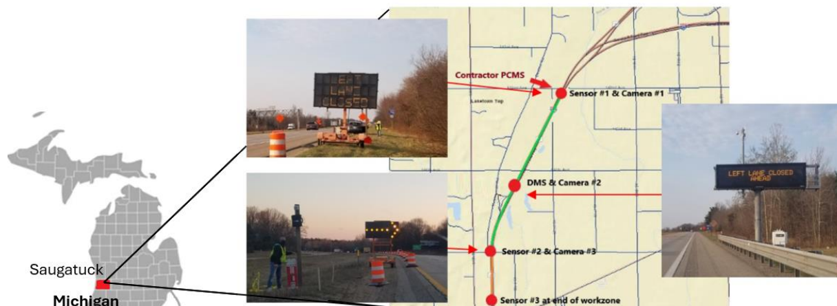
Figure 7. Experiment setup for PCMS work zone-related message
