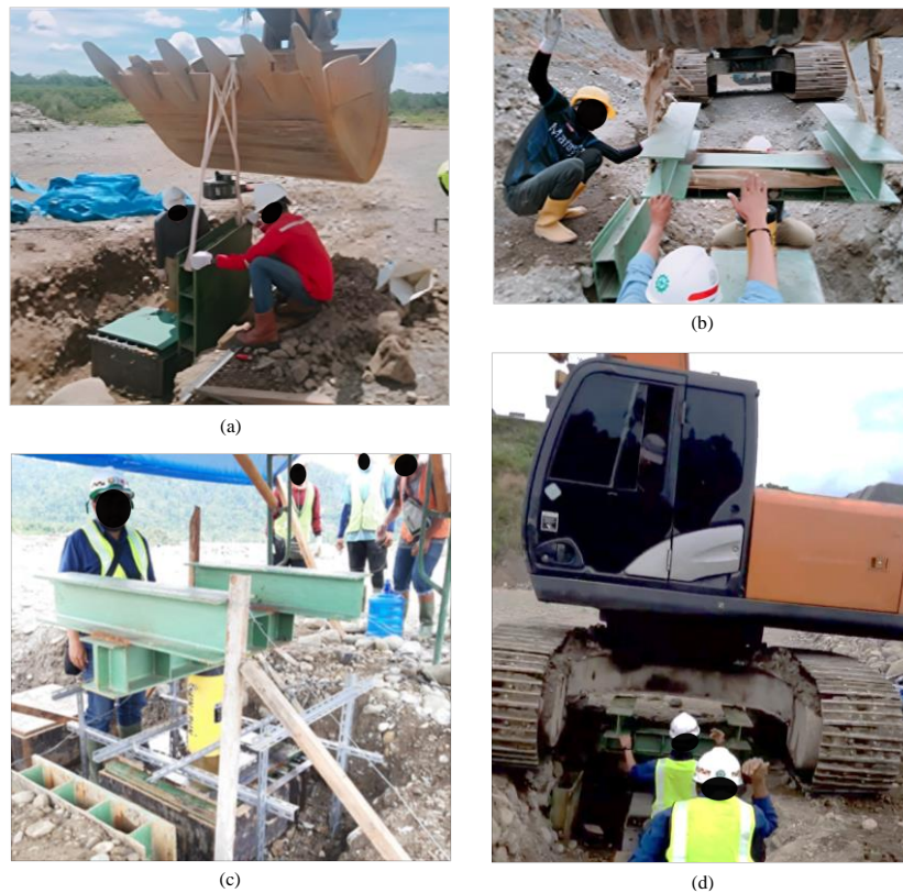
Figure 10. Field test setup: (a) steel plate horizontal reaction, (b) reaction beam installation, (c) hydraulic jack, reference frame, and measuring device installations, and (d) excavator alignment
