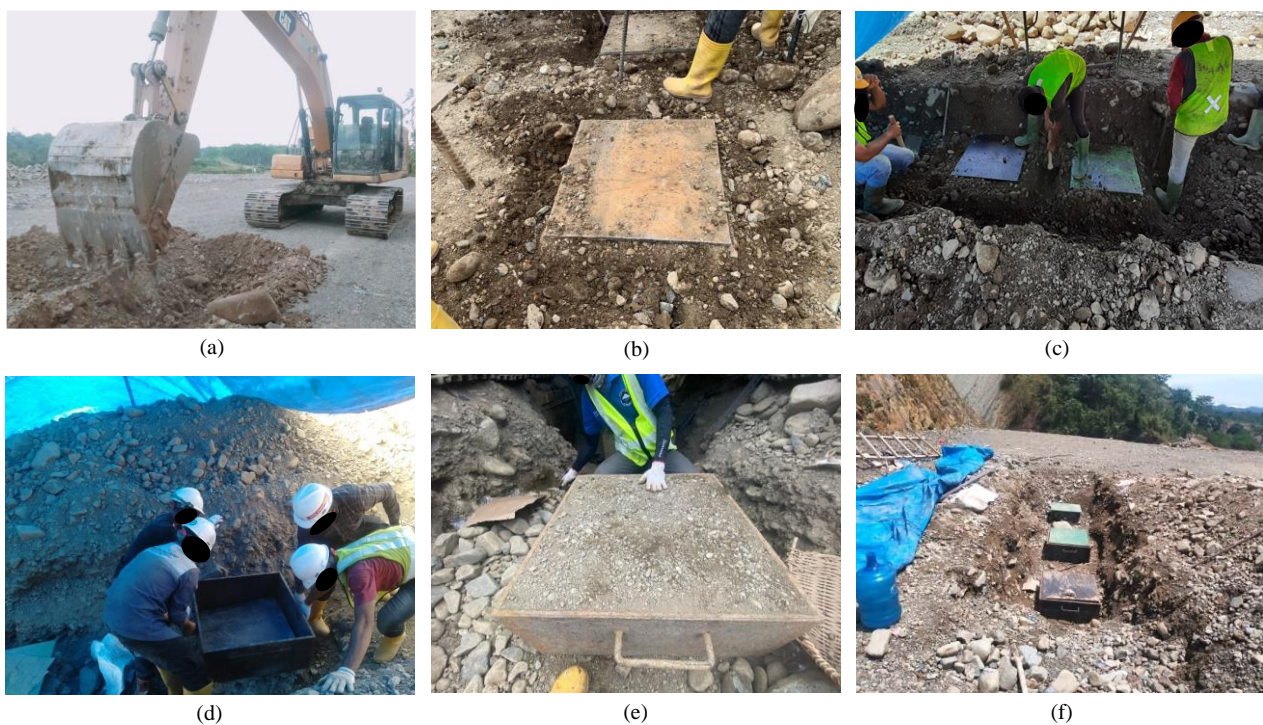
Figure 9. Sample preparation: (a) pit excavation, (b) top plate for template, (c) manual carving, (d) shear box placement, (e) surface sample flattening, and (f) lower top plate installation
