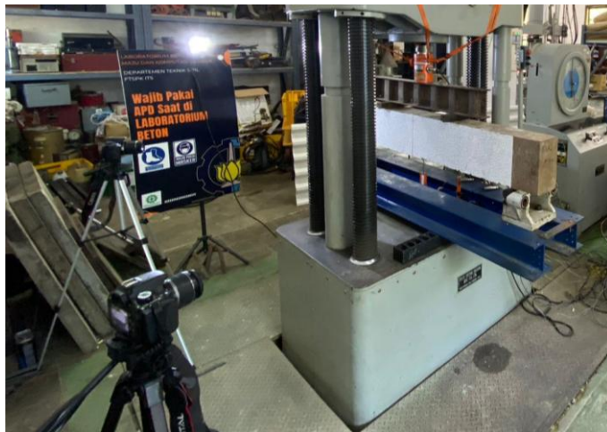
Figure 11. Setup for DIC camera measurements: (a) Camera placement location, (b) Camera placement layout.
