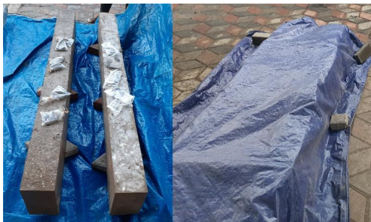
Figure 8. The curing process of the beam specimens
