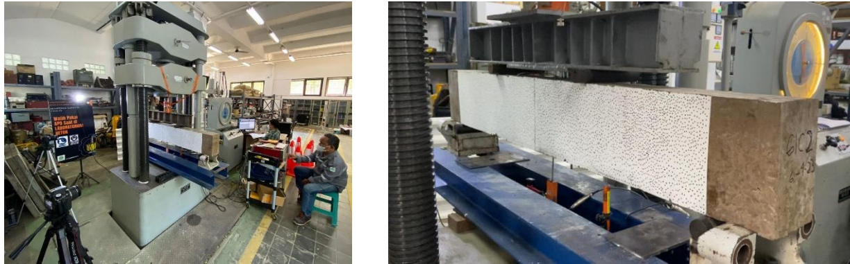
Figure 10. Set up four-point bending testing
