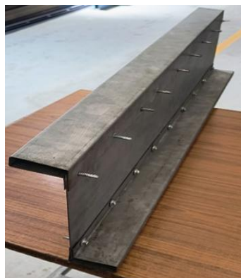
Figure 1. Cold-formed screw-fastened hollow Z-section beam (SFHZ)
