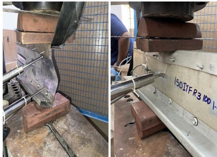
Figure 8. Failure Pattern Analysis in ETF ( Z_1 ) and ITF ( Z_2 ) Experimental Studies
