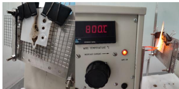
Figure 13. Final glow-wire test results at a test temperature of 800 °C
