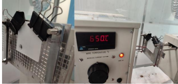
Figure 12. Final glow-wire test results at a test temperature of 650 °C
