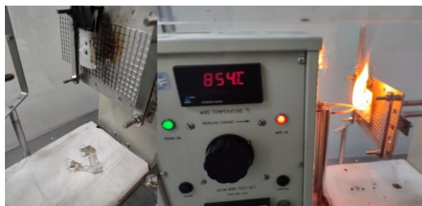
Figure 14. Final glow-wire test results at a test temperature of 850 °C
