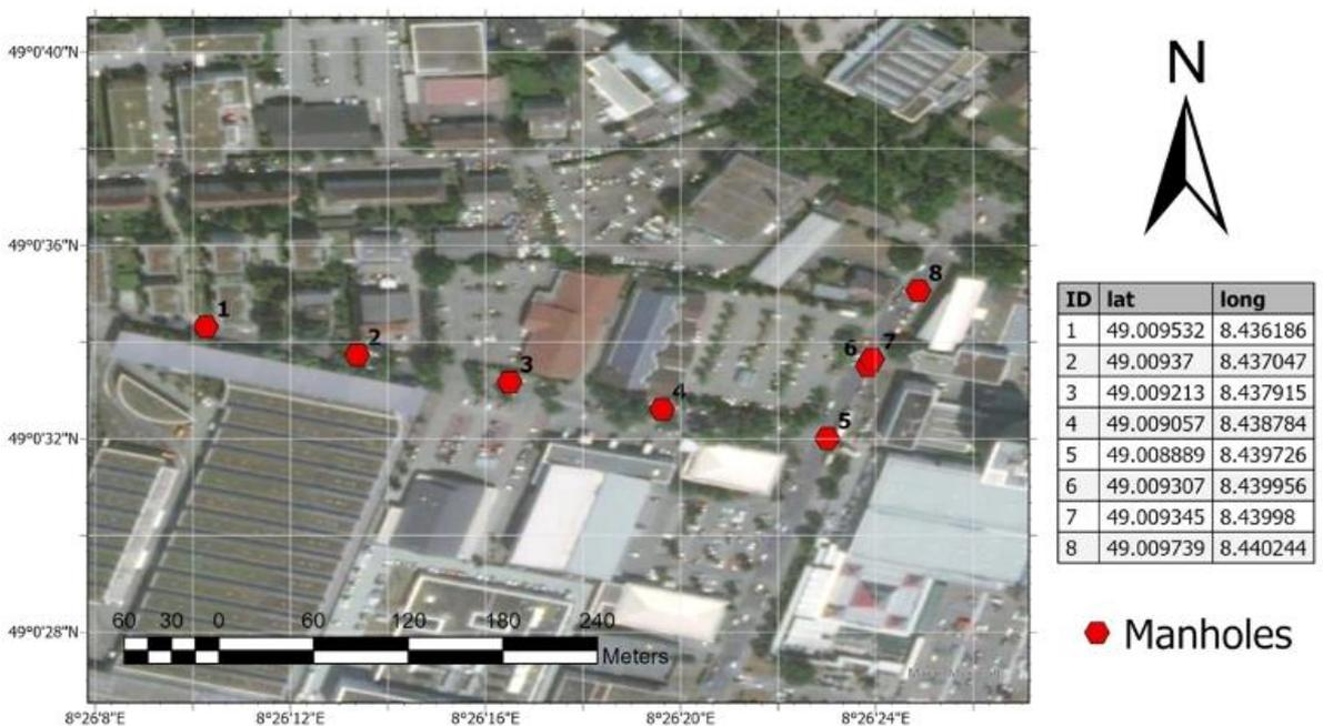
Figure 15. Sequence 9 manhole database on ArcGIS
