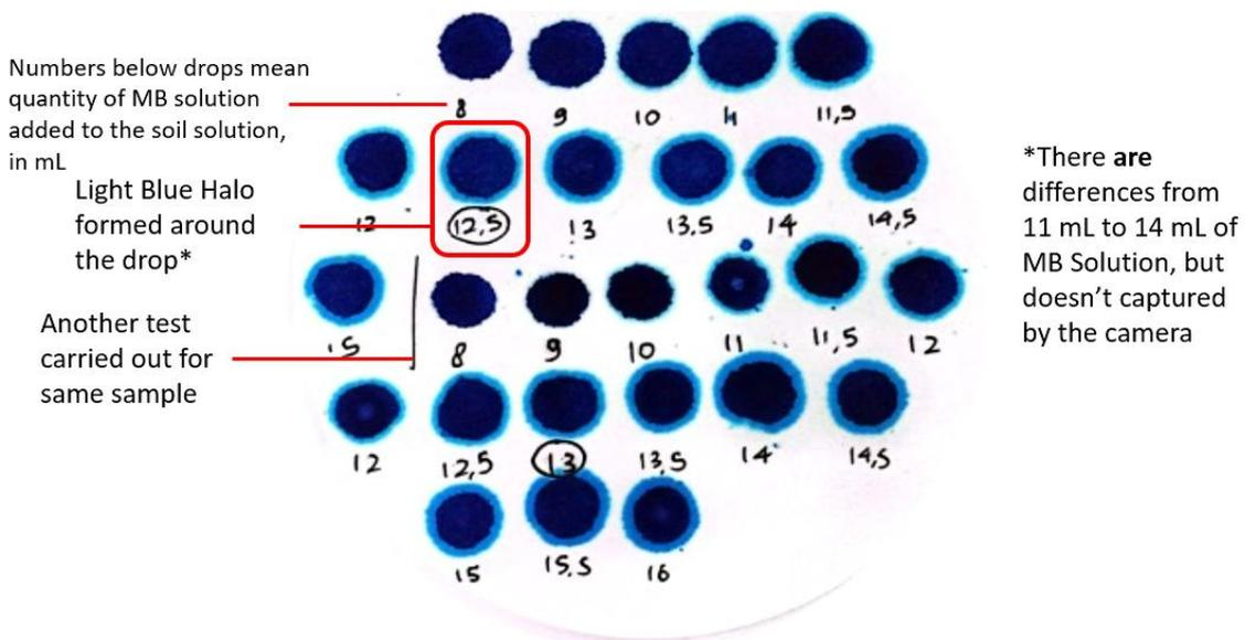
Figure 4. Light blue halo formed in the wet zone of the methylene blue drop
