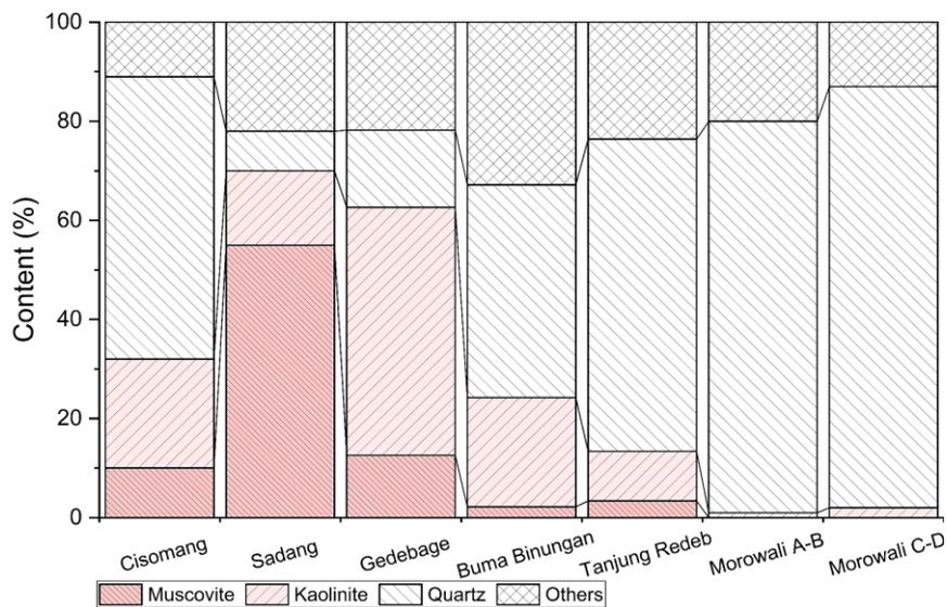
Figure 7. Mineral content from XRD test for each sample
