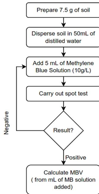
Figure 5. Methylene blue test procedure
