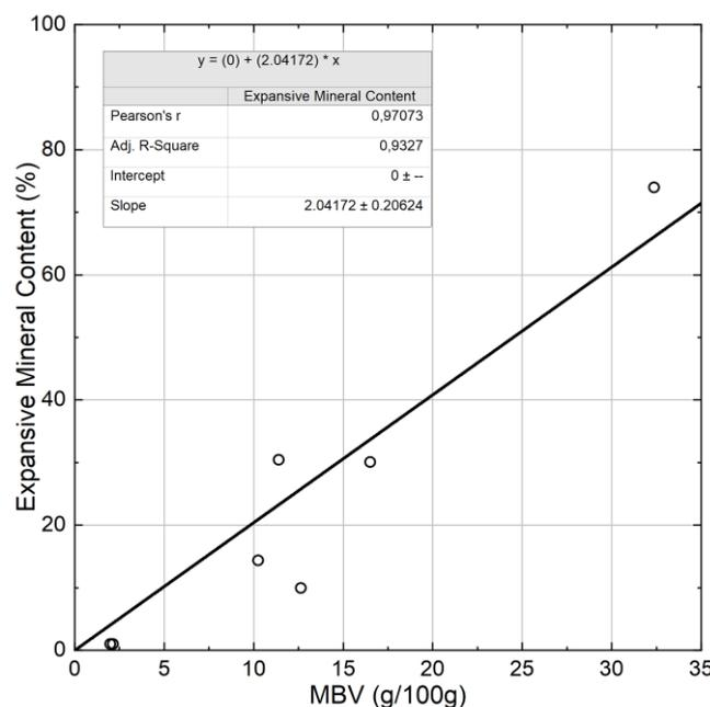
Figure 11. Expansive Mineral Content vs. Methylene Blue Value Regression
