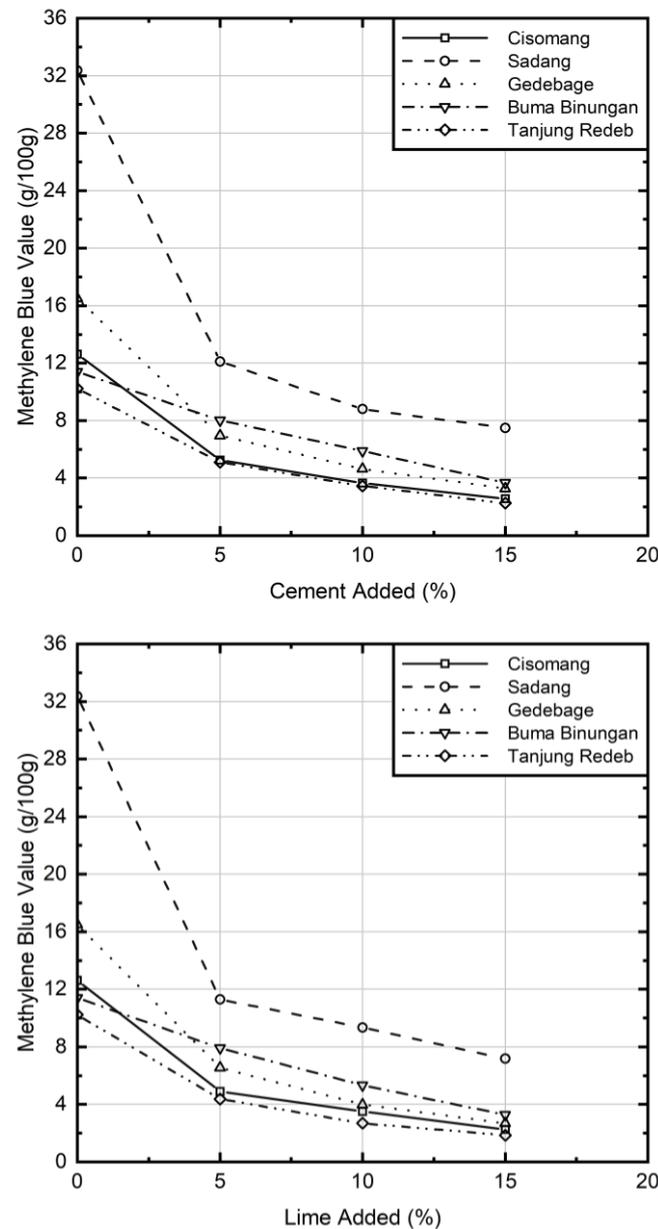
Figure 9. Methylene Blue Test result
