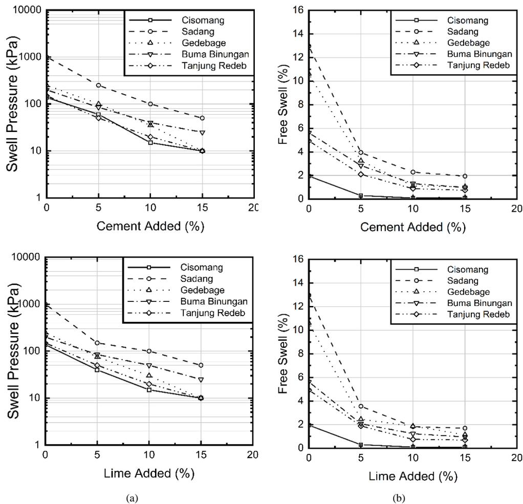
Figure 8. Swell test result in soil parameters (a) swell pressure, and (b) free swell
