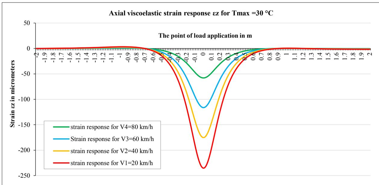
Figure 12. The viscoelastic strain results relative to speed variations for  $T_{max}= 30\text{ }^\circ\text{C}$
