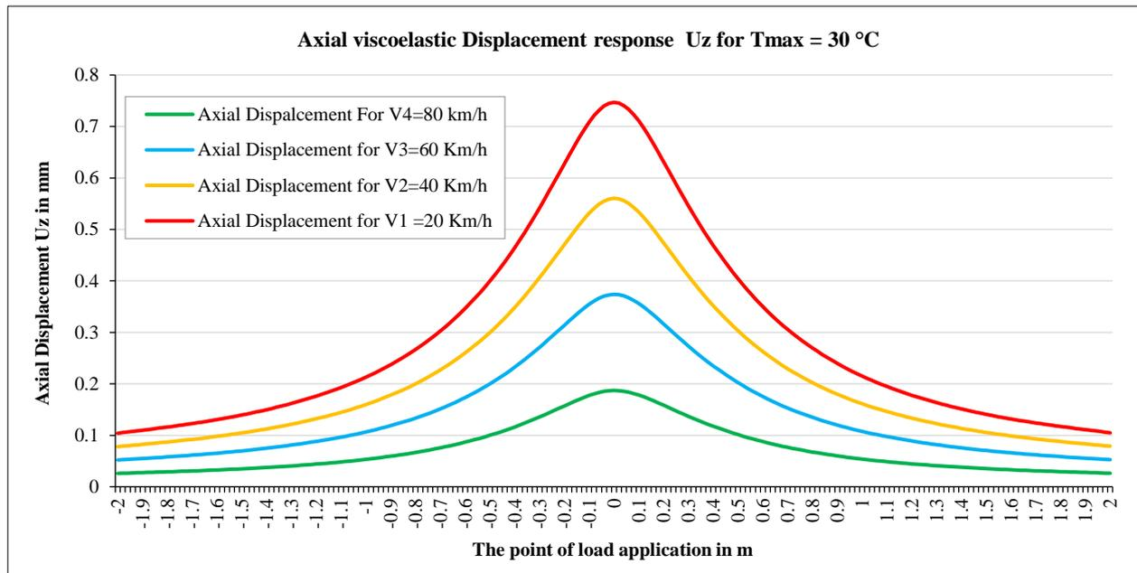
Figure 13. The axial viscoelastic displacement  $U_z$  for  $T_{max} = 30\text{ }^\circ\text{C}$
