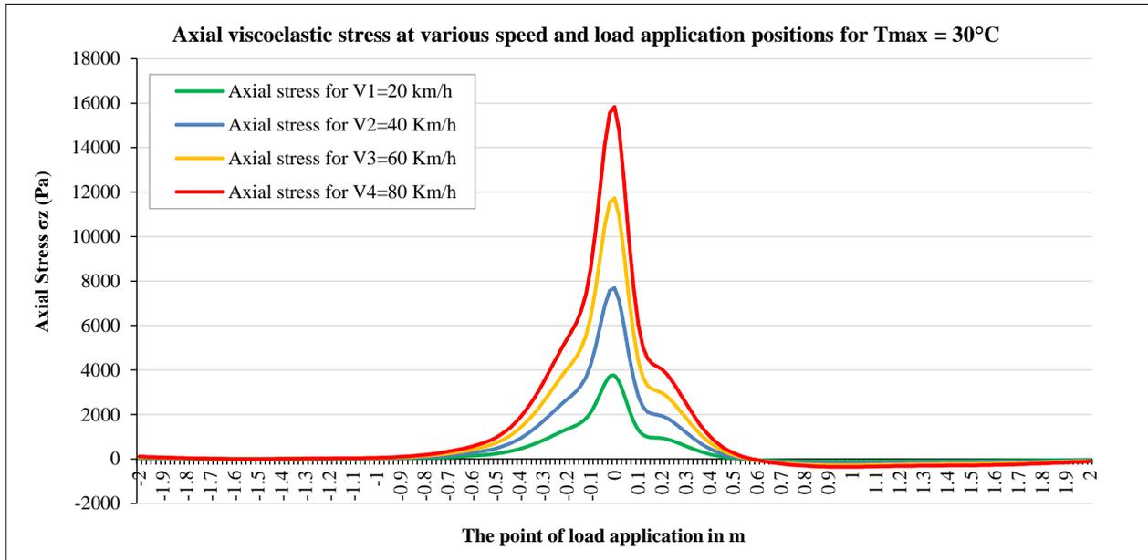
Figure 11. The viscoelastic stress results for  $T_{max} = 30\text{ }^\circ\text{C}$
