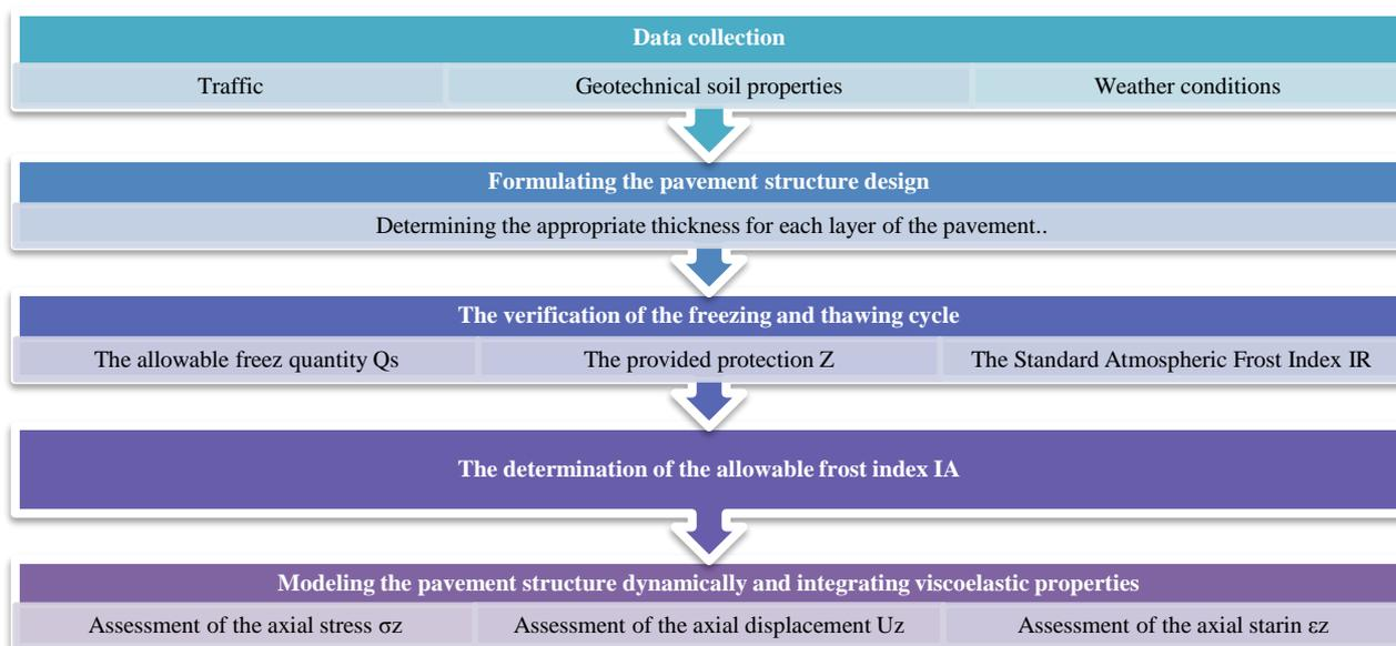
Figure 1. The flowchart outlines the methodology implemented in the research
