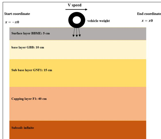
Figure 7. The adopted pavement structures
