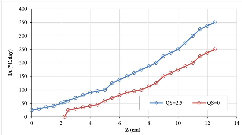
Figure 5. The allowable frost index IA as a function of Z
