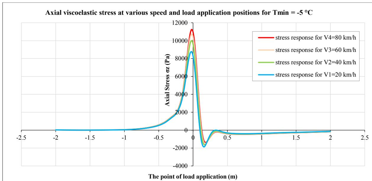
**Figure 8. The viscoelastic stress results for Tmin= -5 °C**
