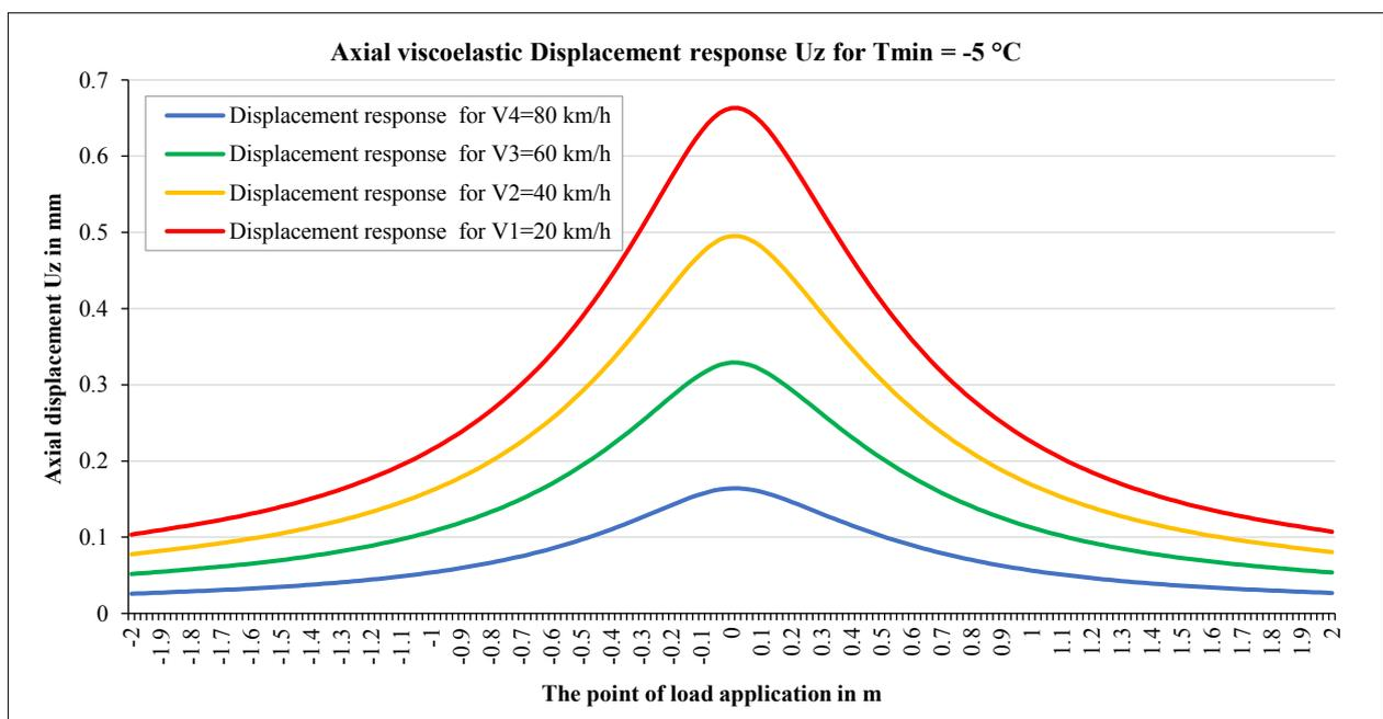
Figure 10. The axial viscoelastic displacement  $U_z$  for  $T_{min} = -5^{\circ}C$
