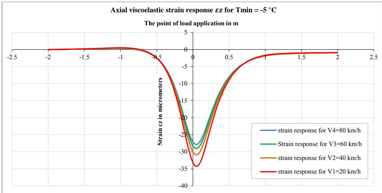
Figure 9. The viscoelastic strain results relative to speed variations for  $T_{min} = -5^{\circ}C$
