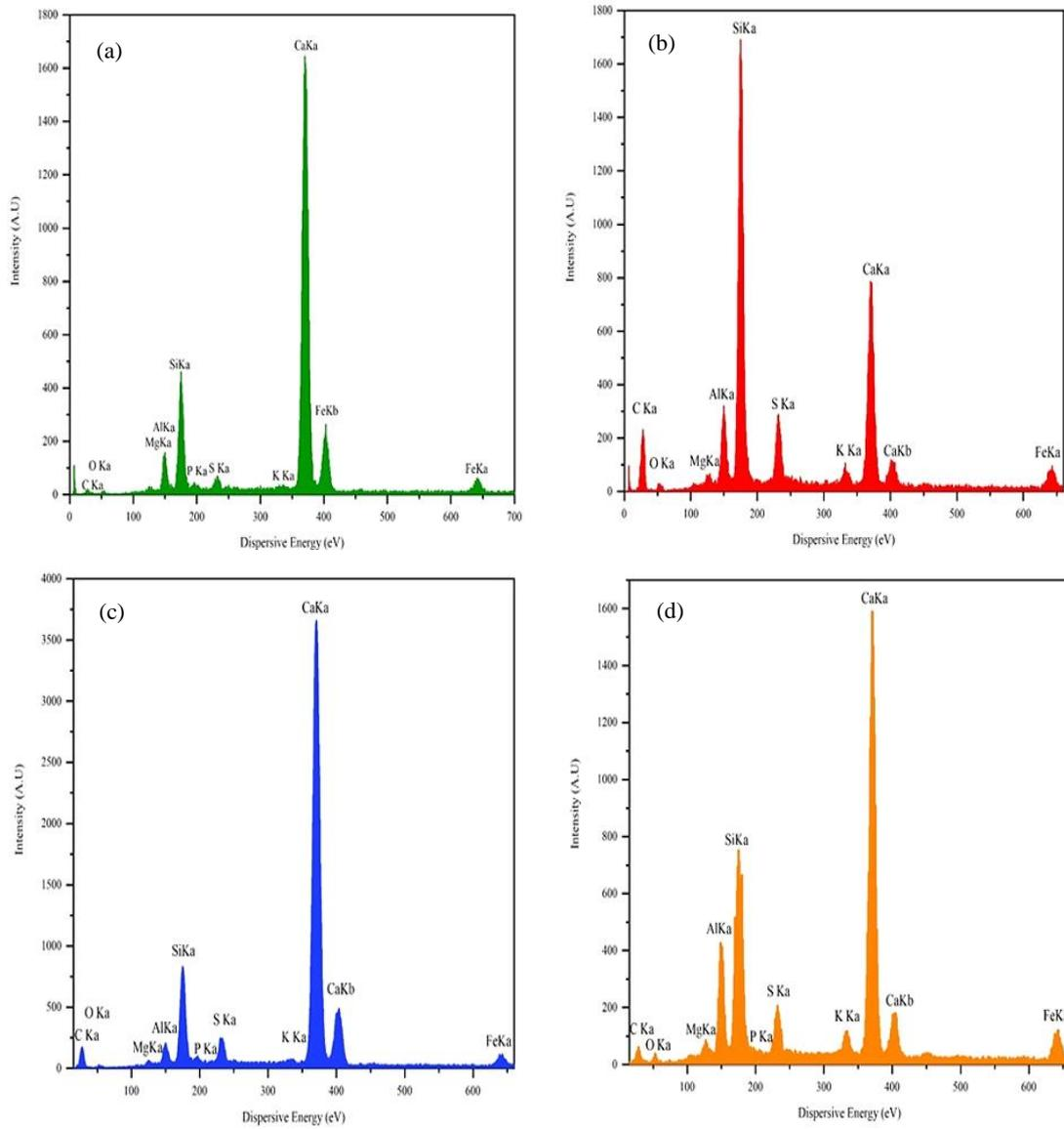
Figure 8. EDAX spectra of (a) CM, (b) 0, (c) 12 and (d) 24 Months treated RAP in Pervious Concrete
