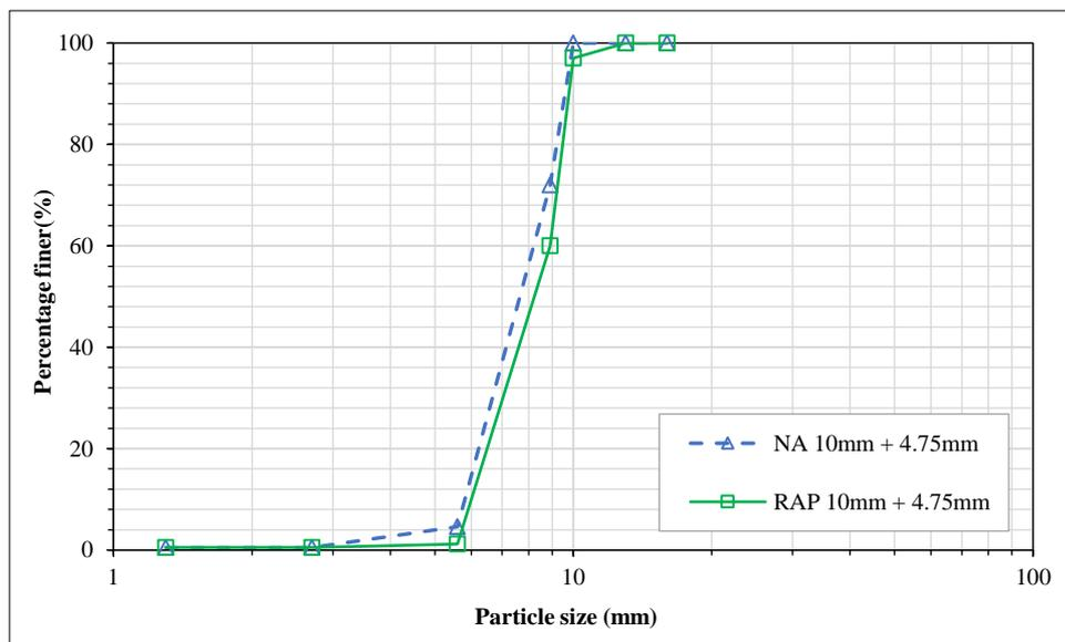
**Figure 4. Grain sieve analysis of Natural Aggregate and RAP**
