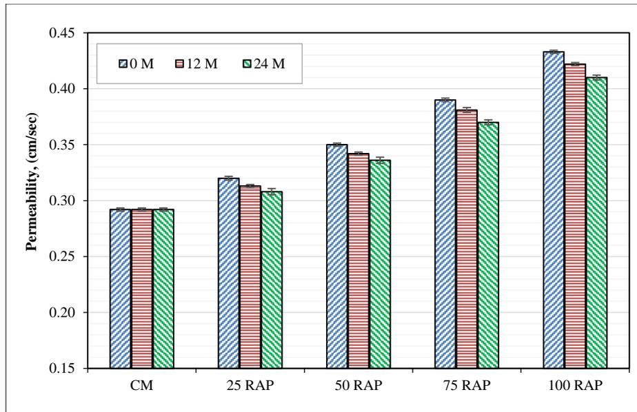
Figure 10. Permeability of Pervious Concrete with 0, 12, and 24 Months Treated RAP
