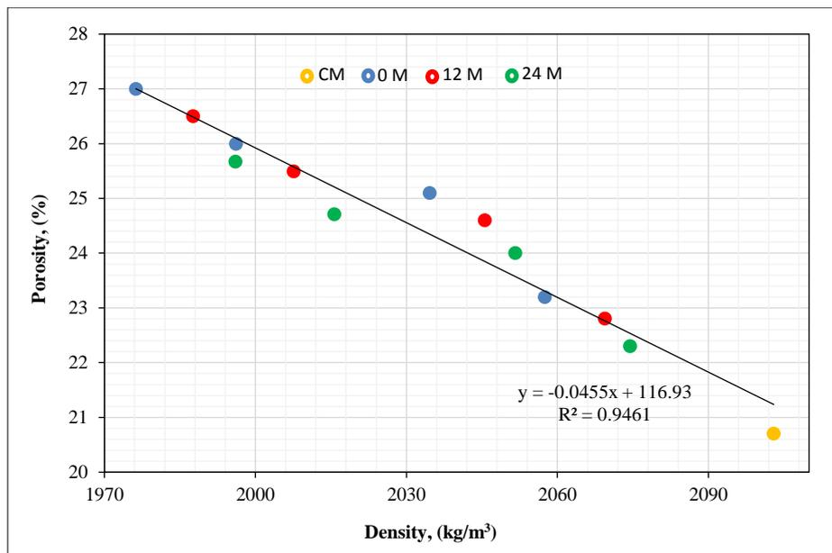
Figure 9. Comparative analysis of porosity and density trends in pervious concrete containing RAP at different treatment durations
