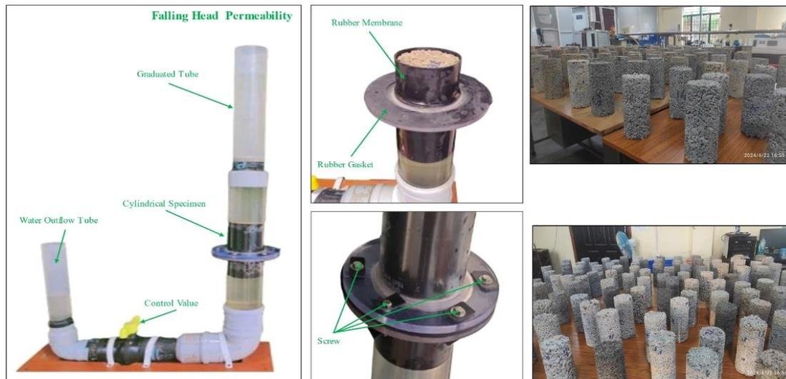
Figure 5. In-House Permeability Test Setup and samples
