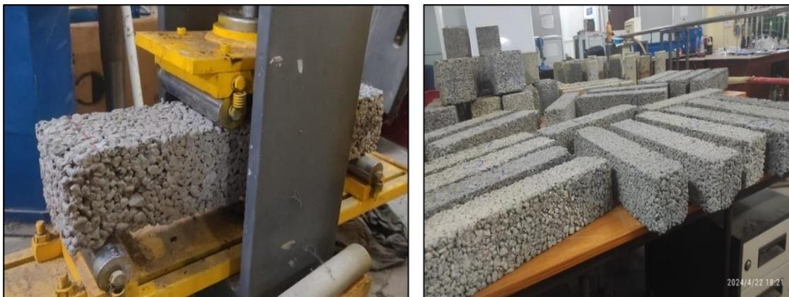
Figure 13. Flexural Strength of Pervious Concrete with Treated RAP
