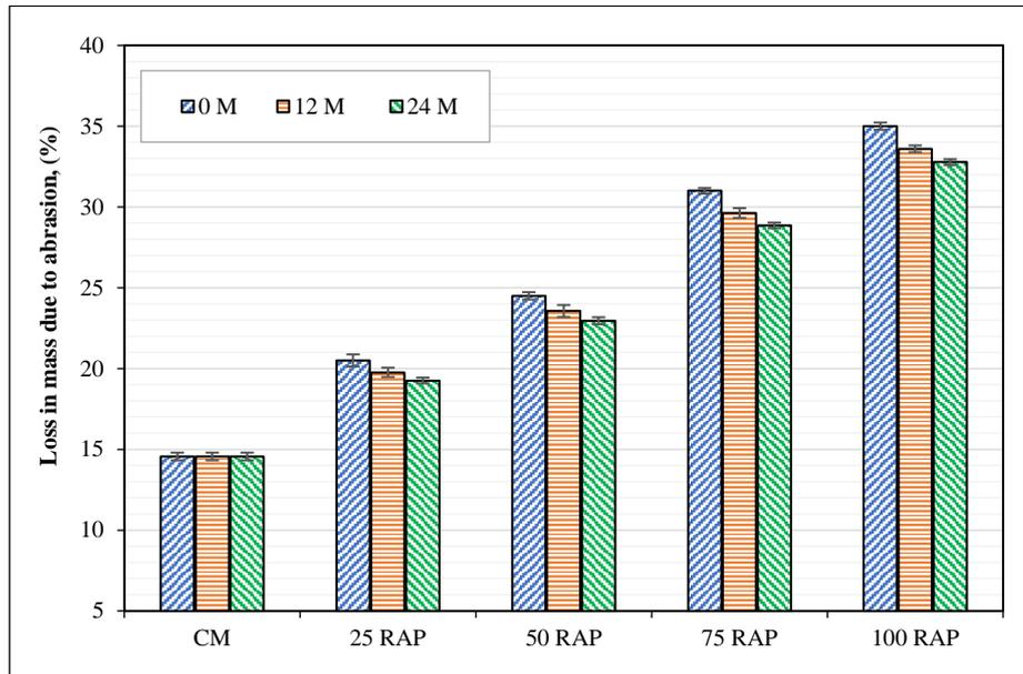
Figure 15. Mass Loss from Abrasion in Pervious Concrete with 0, 12, and 24 Months Treated RAP
