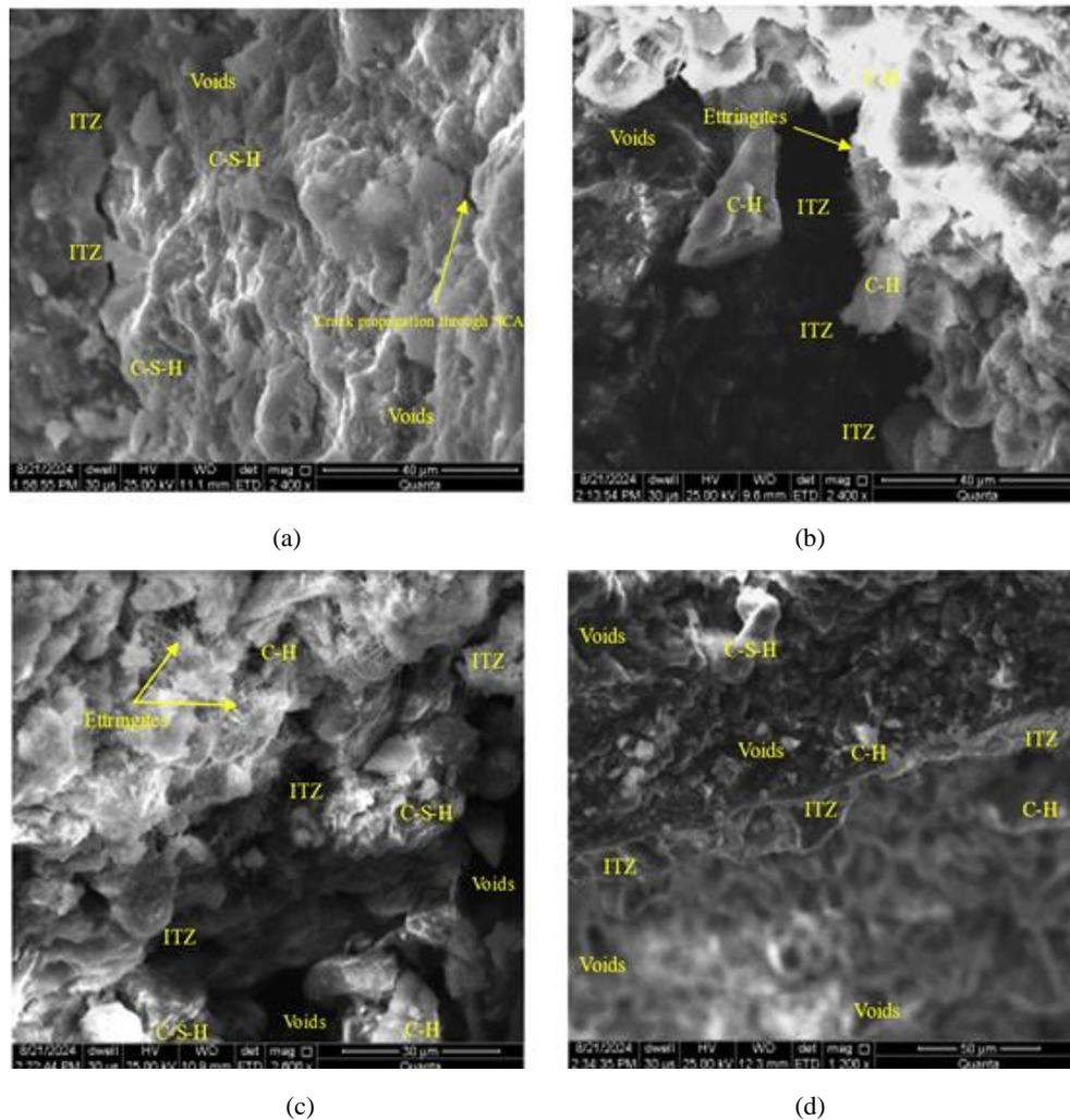
Figure 7. SEM images of (a) CM, (b) 0, (c) 12 and (d) 24 months treated RAP in Pervious concrete
