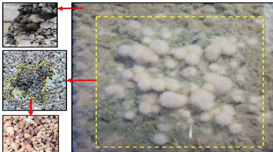
Figure 18. Formation of ettringites on soaking PC in H<sub>2</sub>SO<sub>4</sub> acid
