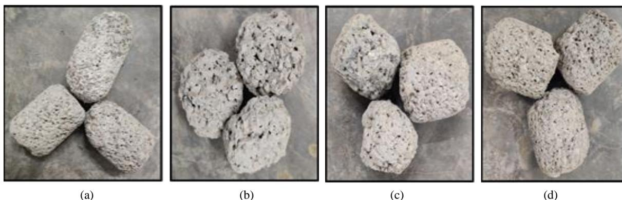
Figure 16. Abraded specimens of (a) CM, (b) 0 Month, (c)12 Months and (d) 24 Month Treated RAP incorporated PC
