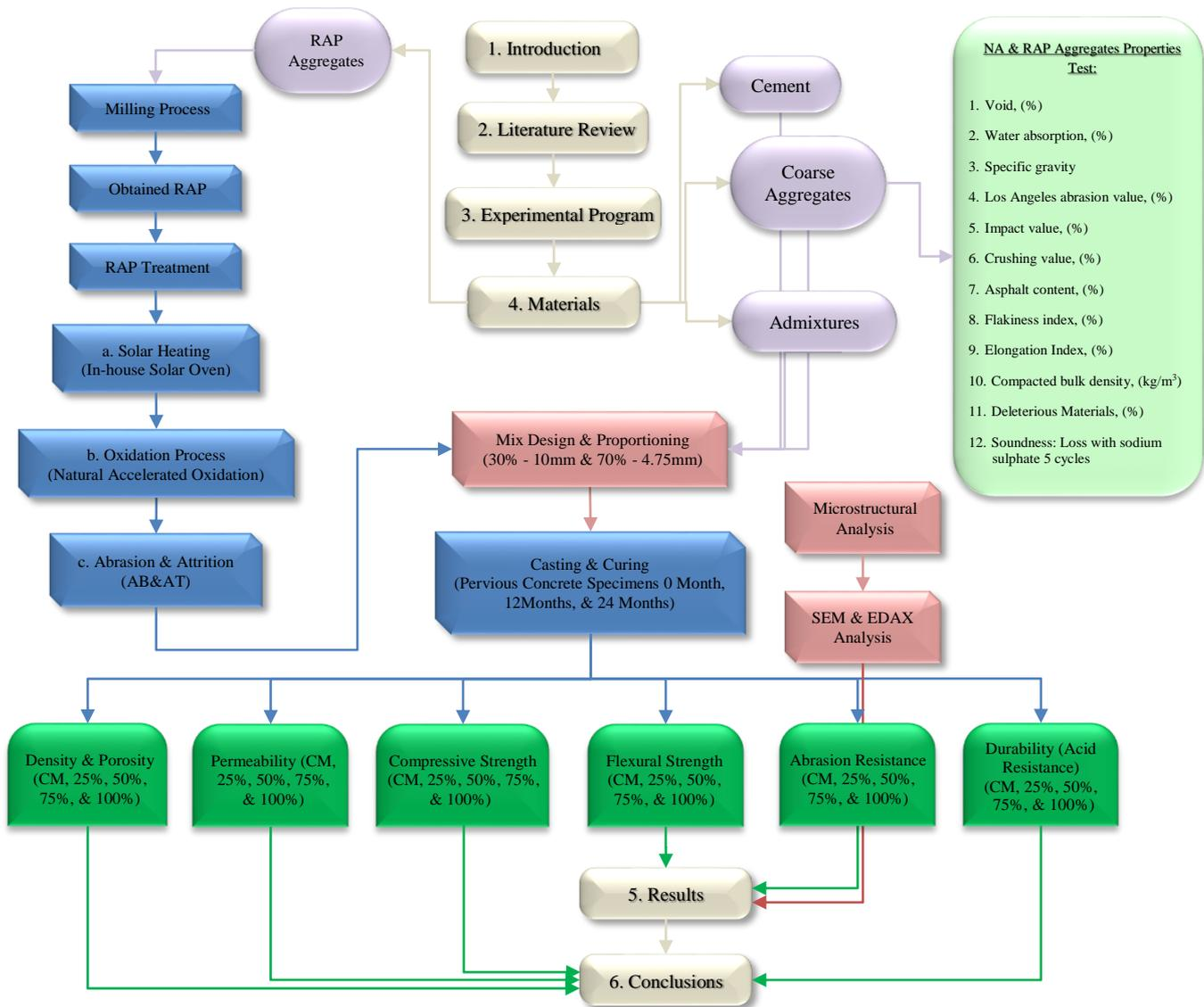
Figure 1. Process flow diagram of the methodology used in this research
