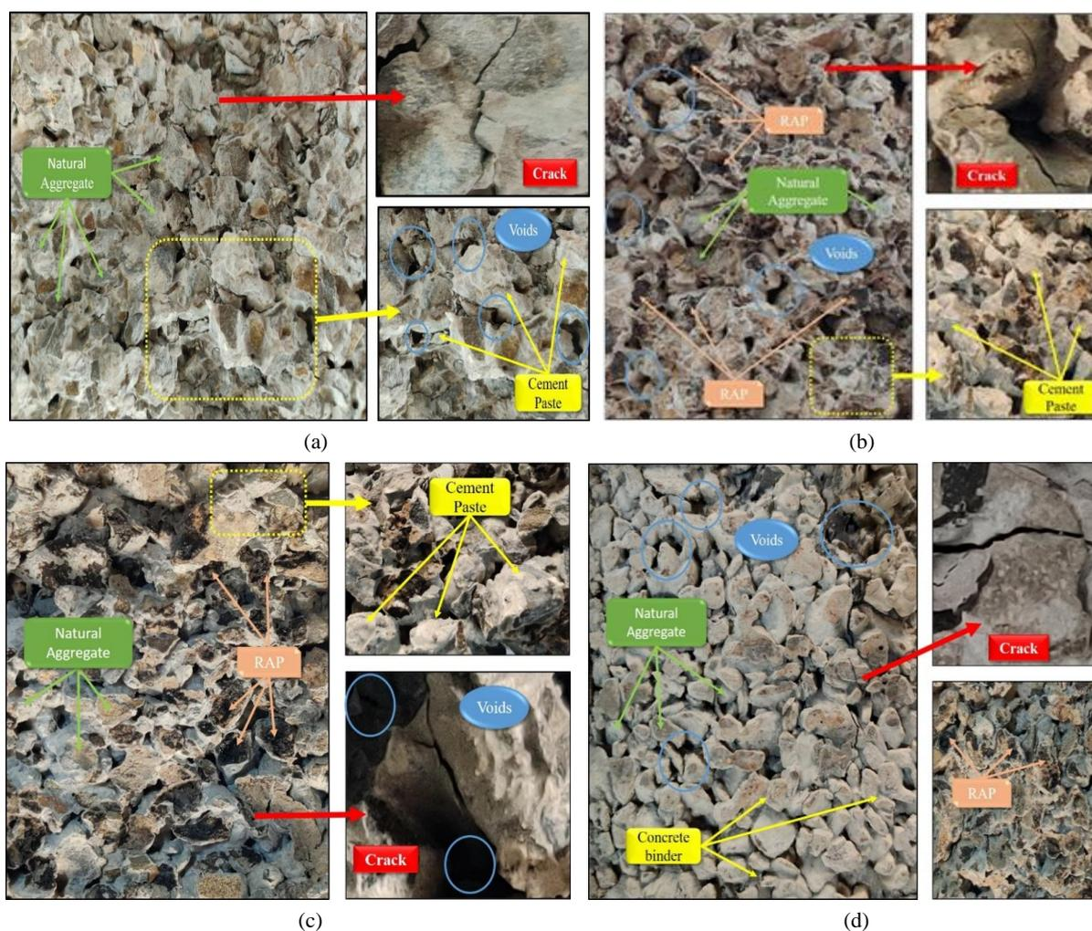
Figure 19. (a) CM, (b) 0 Month, (c) 12 Months and (d) 24 Months pre-treated RAP aggregate concrete
