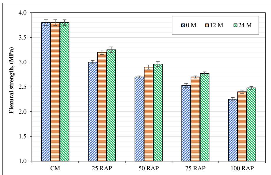
Figure 14. Flexural Strength of Pervious Concrete with 0, 12, and 24 Months Treated RAP
