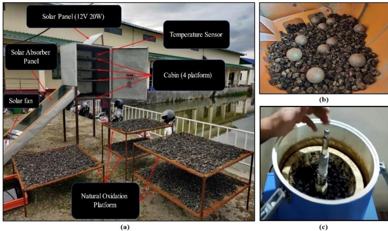
Figure 2. (a) The Solar oven for heating the RAP (b) Abrasion and Attrition (AB&AT) (c) Bitumen Extraction Test of RAP
