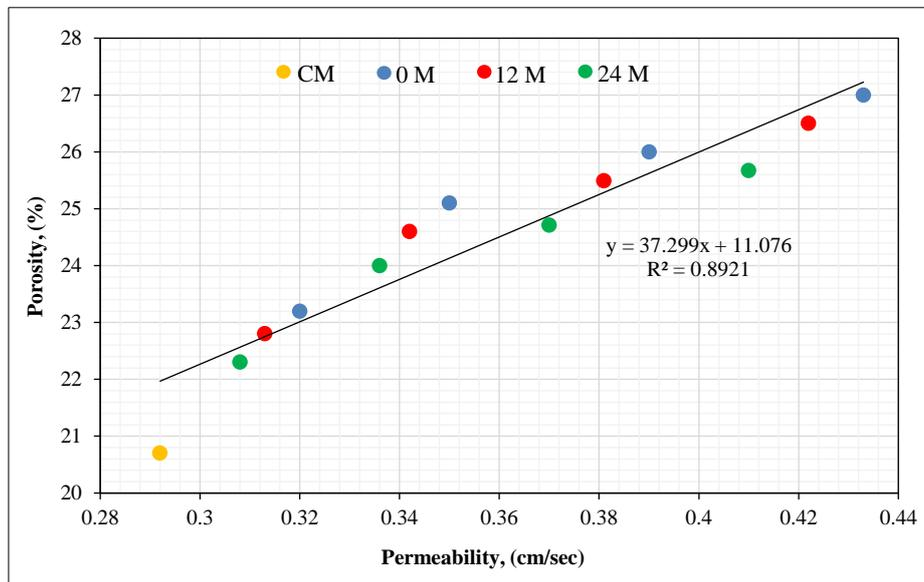
Figure 11. Relationship between porosity and permeability in pervious concrete incorporating RAP treated for 0, 12, and 24 months
