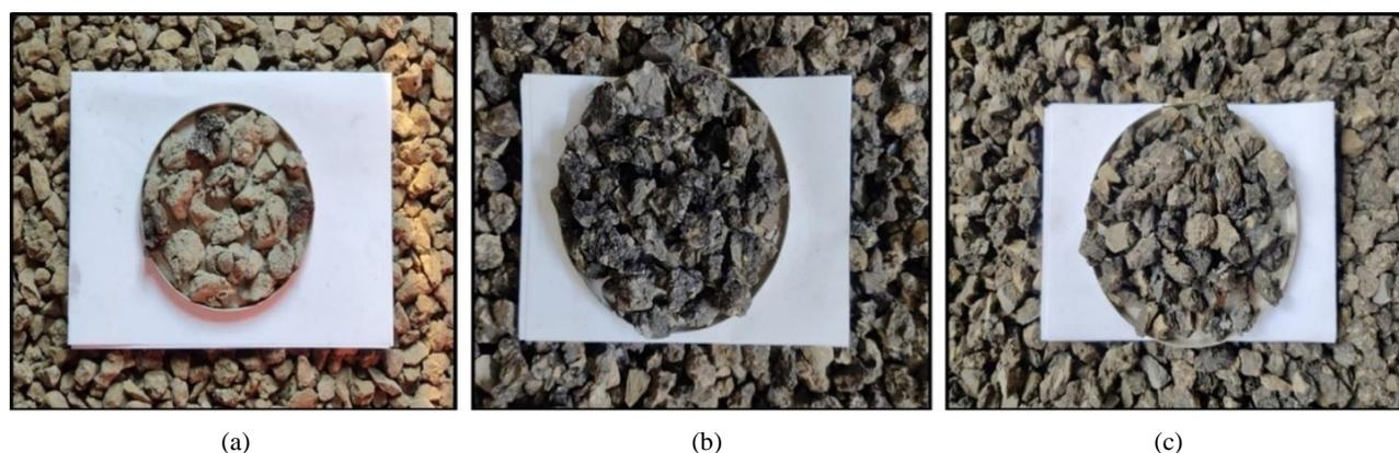
Figure 3. RAP Samples after (a) 0, (b) 12, and (c) 24 Months of Treatment
