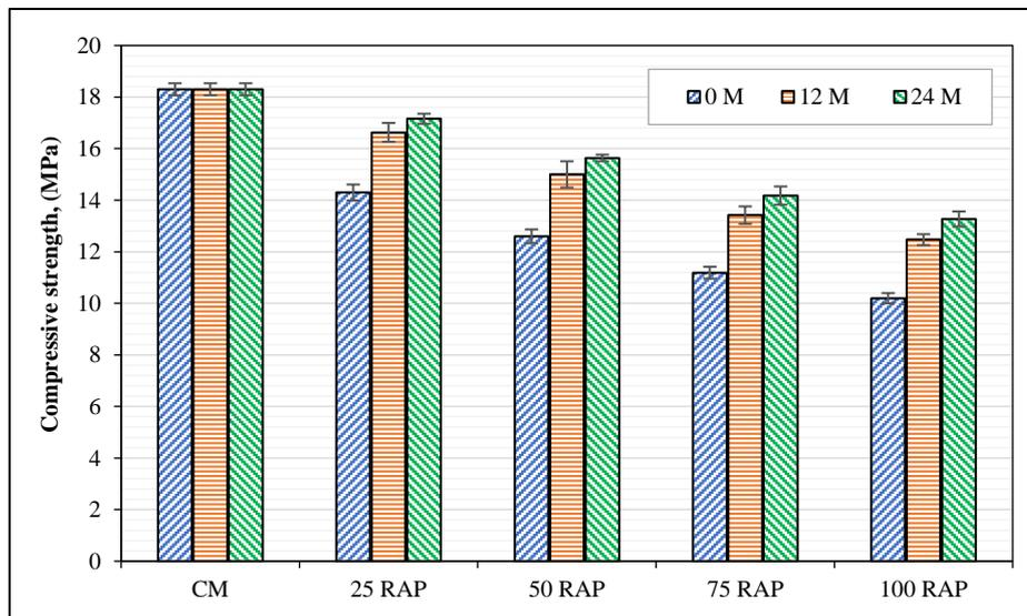
Figure 12. Compressive Strength of Pervious Concrete with 0, 12, and 24 Months Treated RAP
