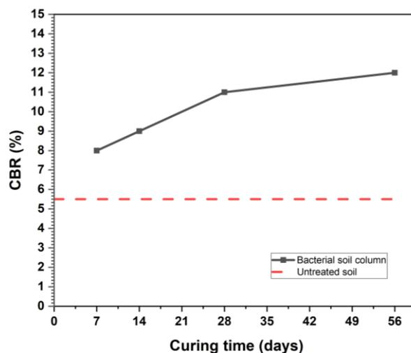
Figure 9. Relationship between curing time and CBR value of bacterial soil column
