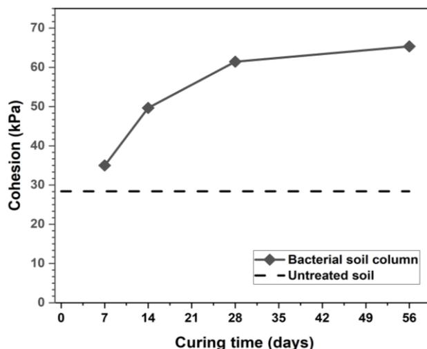
**Figure 15. Relationship between curing time and average cohesion value of bacterial soil column**
