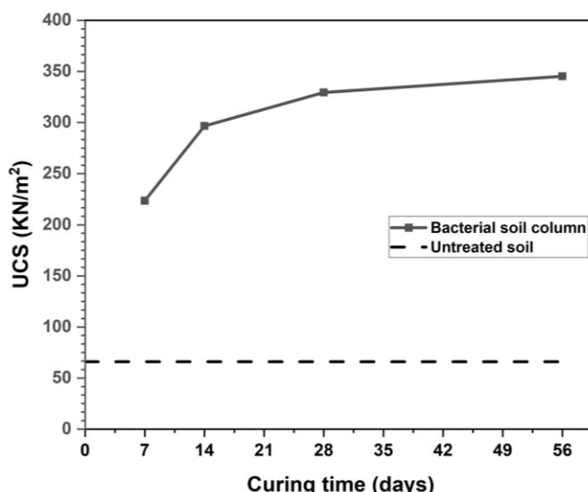
Figure 13. Relationship between curing time and the average value UCS of the bacterial soil column
