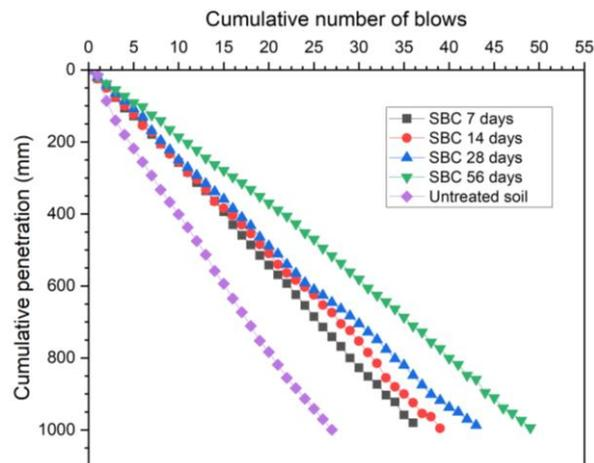
Figure 8. The relationship between the number of blows and the decrease based on the curing time
