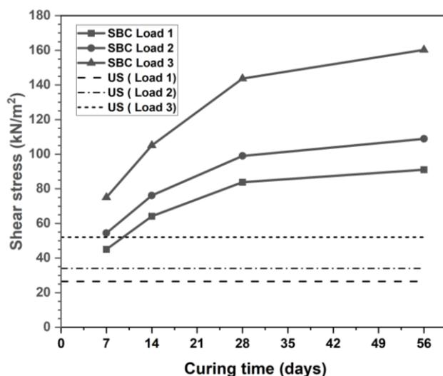
Figure 18. Relationship between curing time and average shear stress in the column of bacterial soil and untreated soil under three different loading conditions
