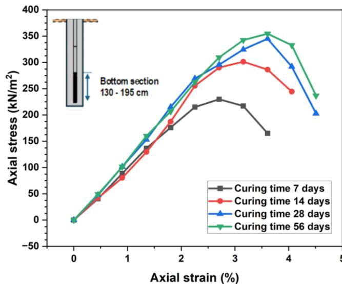
Figure 12. Relationship between axial stress vs. deformation when applied on the bacterial soil column
