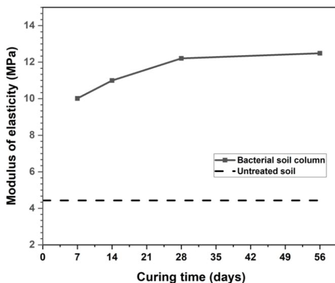
Figure 14. Relationship between curing time and average modulus of elasticity of bacterial soil column
