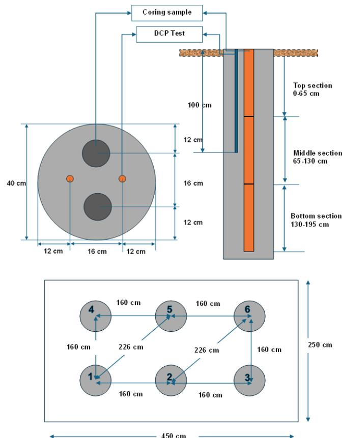
Figure 7. Details on DCP testing and sampling locations
