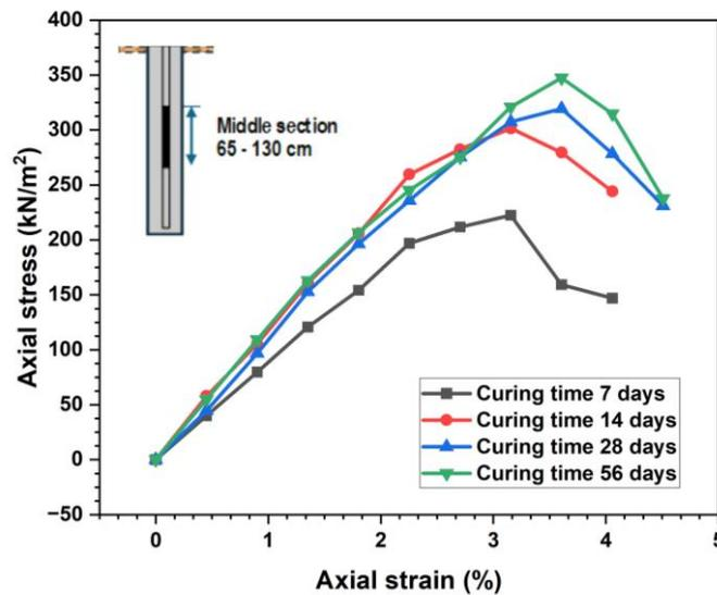
Figure 11. Relationship between axial stress vs. deformation when applied on the bacterial soil column
