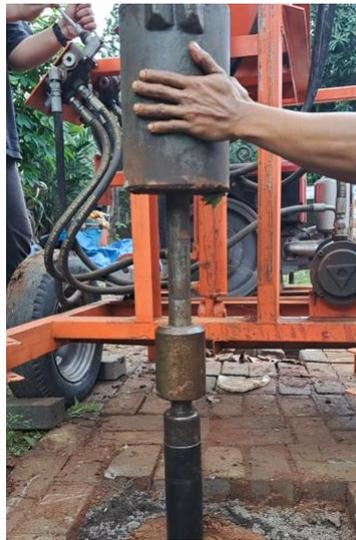
Figure 6. Coring for bacterial soil sampling
