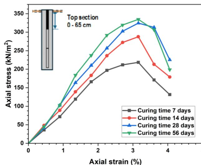
**Figure 10. Relationship between axial stress vs. deformation when applied on the bacterial soil column**
