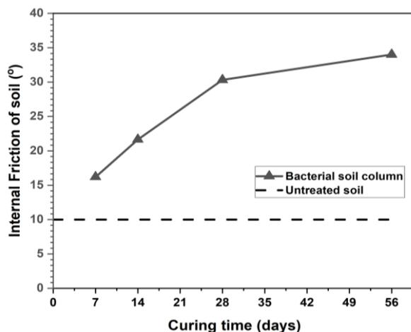
Figure 16. Relationship between curing time and average internal friction angle of the bacterial soil column
