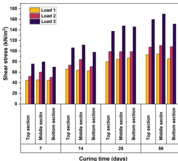
Figure 17. Relationship between curing time and shear stress in bacterial soil columns divided into three sections under three different loading conditions
