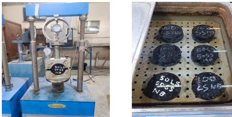
Figure 3. Marshall test equipment and the specimens in water path at 60°C (ASTM D6926-20) before test
