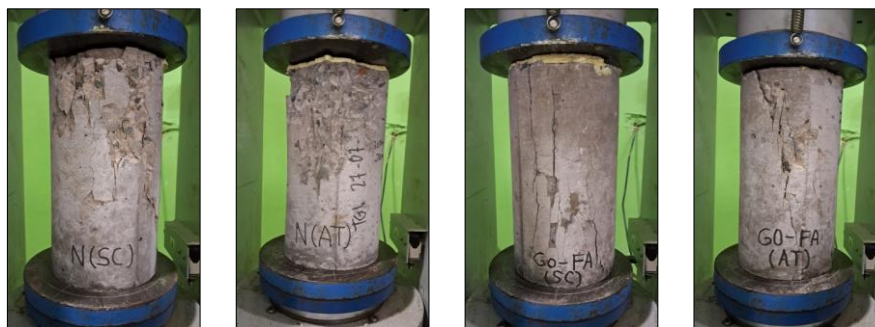
Figure 9. Concrete specimen failures at 28-day compression testing (a) Control concrete under standard curing (b) Control concrete under ambient temperature (c) GO-FA concrete under standard curing (d) GO-FA concrete under ambient temperature
