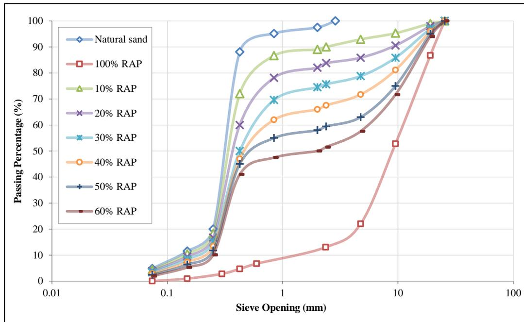
Figure 5. Gradation curves of sand-RAP mixtures
