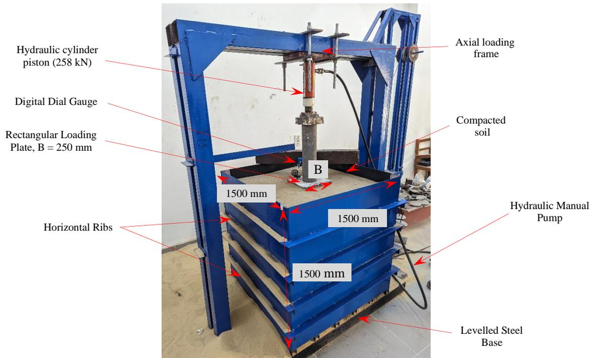
Figure 4. Experimental soil tank and test setup
