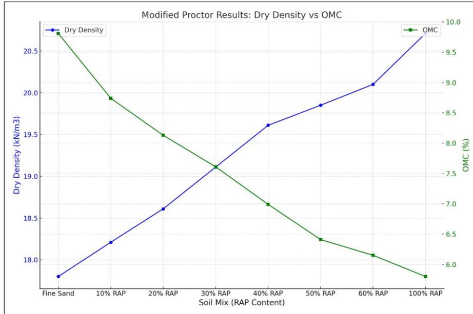
Figure 12. RAP-sand blends' maximal dry density and OMC
