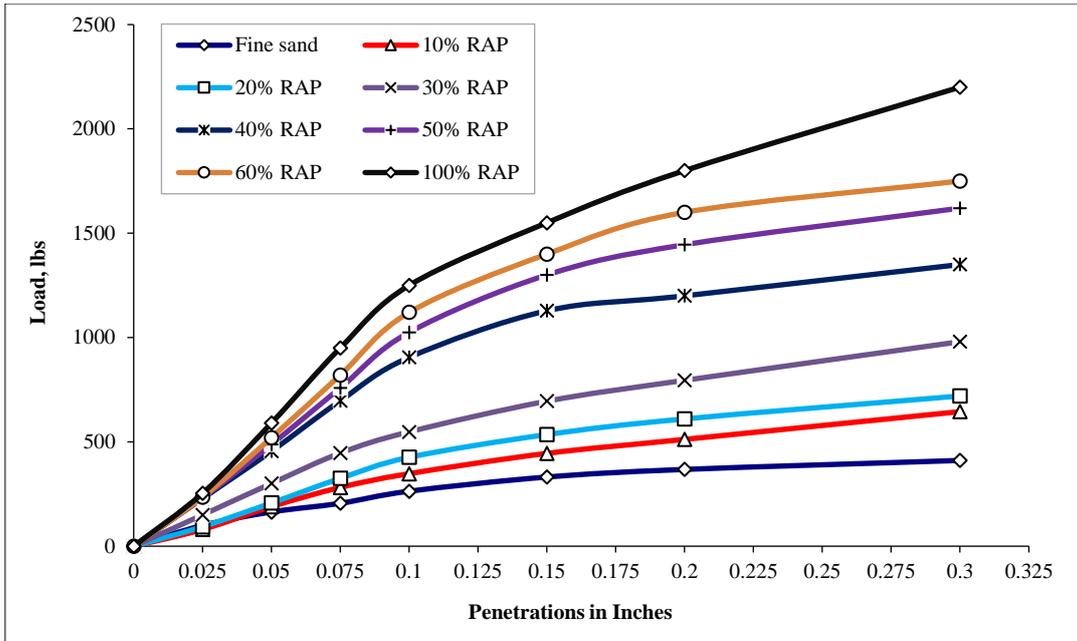
Figure 6. Load penetration curve for RAP-sand mixtures (CBR results)
