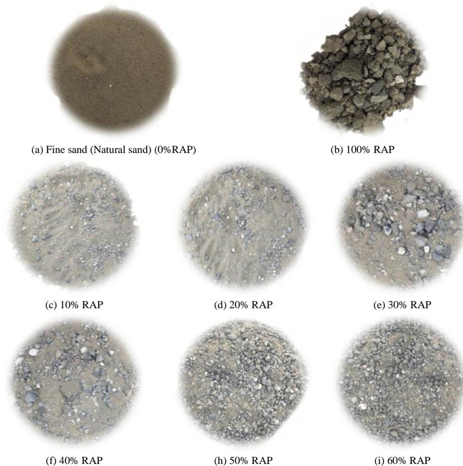
**Figure 2. Images of sand-RAP mixtures with varying RAP proportions (R: 0%, 10%, 20%, 30%, 40%, 50%, 60%, and 100% by weight)**
