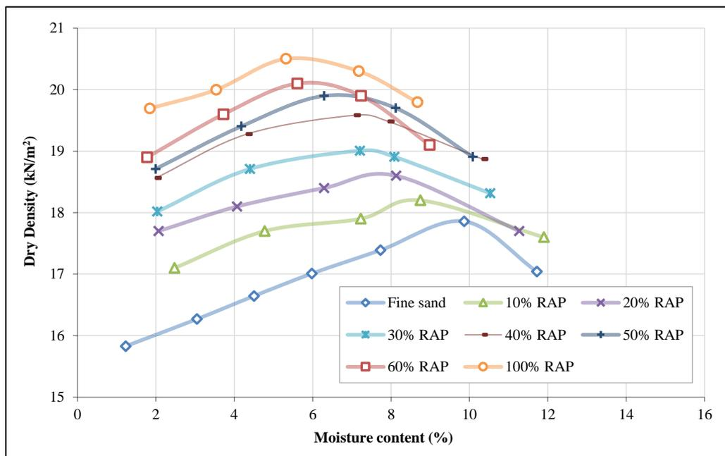
Figure 11. Modified proctor test results for RAP-sand mixtures with varying RAP percentages
