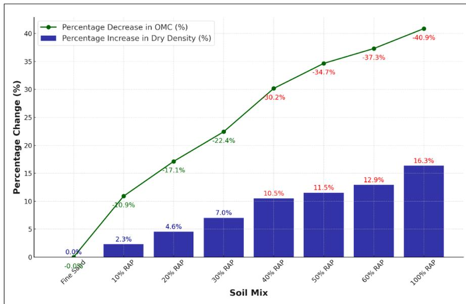
Figure 13. Enhanced compaction indicators as a percentage relative to fine sand
