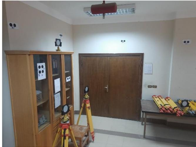
Figure 2. Targets setup
