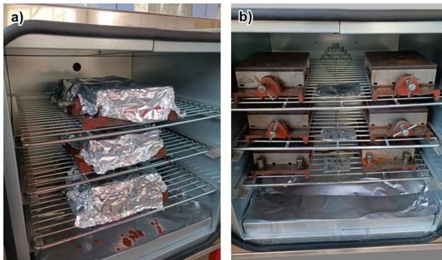
**Figure 5. Curing of alkali-activated mortar samples at 70 °C for 3 days: a) with coverage by foil and b) with coverage by a metal plate**
