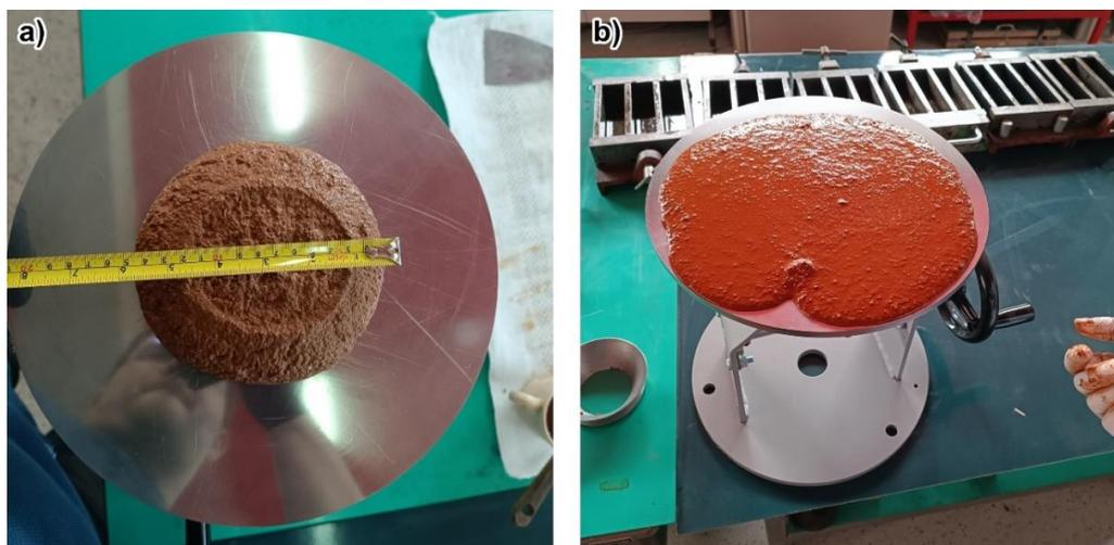
Figure 11. Consistency testing of mortar mixtures: a) plastic consistency and b) fluid consistency
