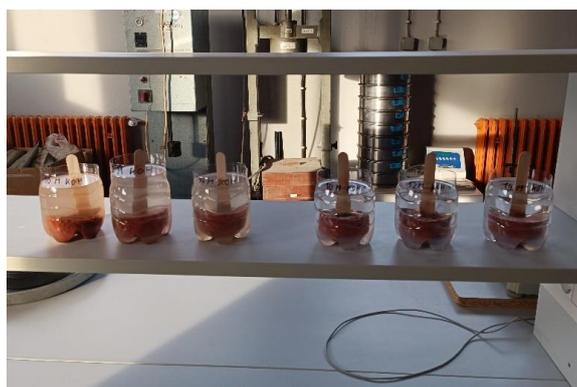
Figure 4. Alkali-activated “lollipops” immersed in water
