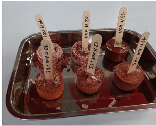
Figure 9. Appearance of alkali-activated “lollipops” cured at elevated temperature
