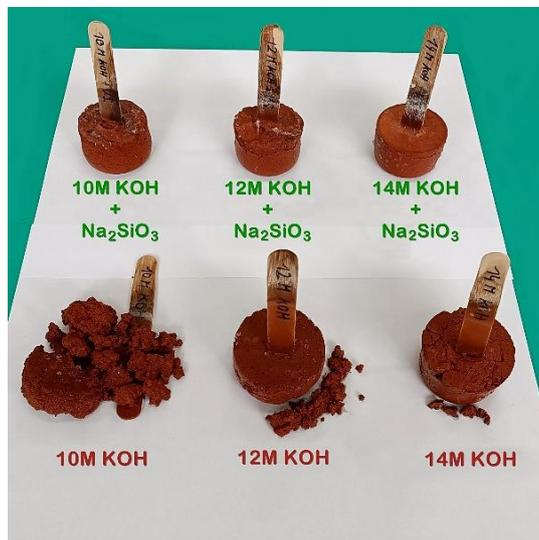
Figure 10. Alkali-activated “lollipops” after 7 days in water
