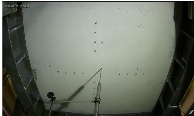
Figure 5. LVDT positioning under the slab to measure the vertical deflection
