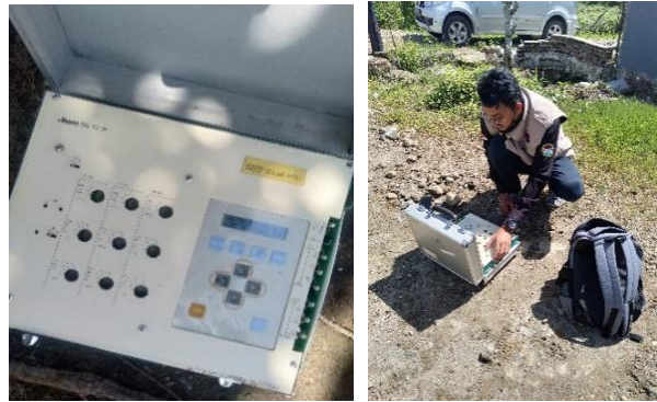
Figure 6. Microtremor GPL-6A3P Sensor (left), field survey (right)
