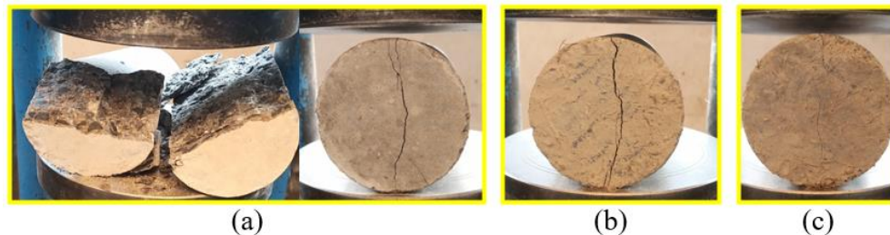
Figure 14. Failure modes of cylinder specimens: (a) control concrete cylinder, (b) concrete cylinder with low fiber content, and (c) concrete cylinder with high fiber content
