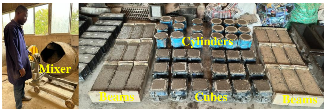
Figure 6. Concrete cast into cube, cylinder, and beam specimens
