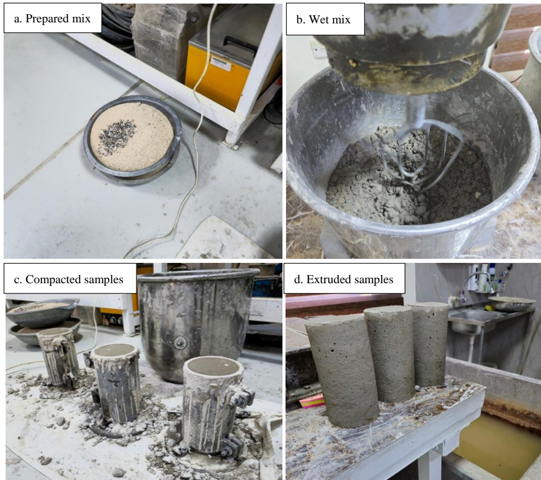
Figure 5. Sample preparation sequence. a: Prepared mix, b: Wet mix, c: Compacted samples, d: Extruded samples
