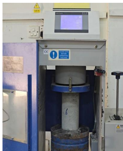
Figure 6. Test Apparatus for Unconfined Compressive Strength Test
