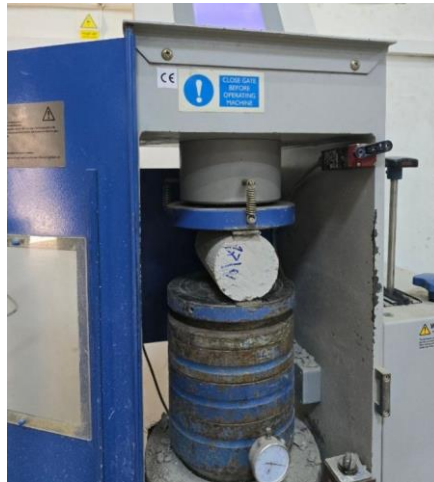
Figure 7. Test Apparatus for Splitting Tensile Strength Test
