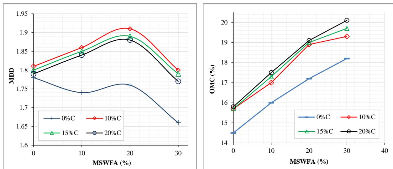
Figure 10. Effect of Cement on the MDD and OMC of Soil-MSWIFA Mix
