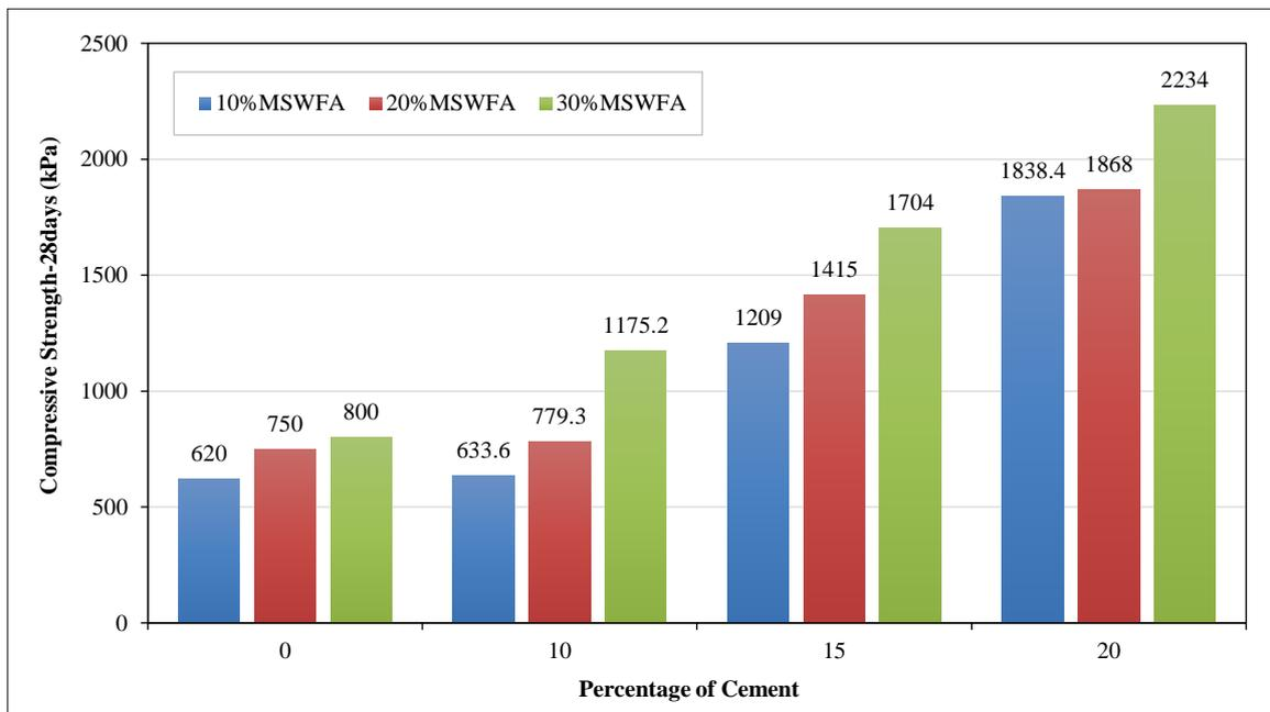
Figure 12. Compressive strength (28 days) of mixtures versus MSWIFA content for different percentages of Cement
