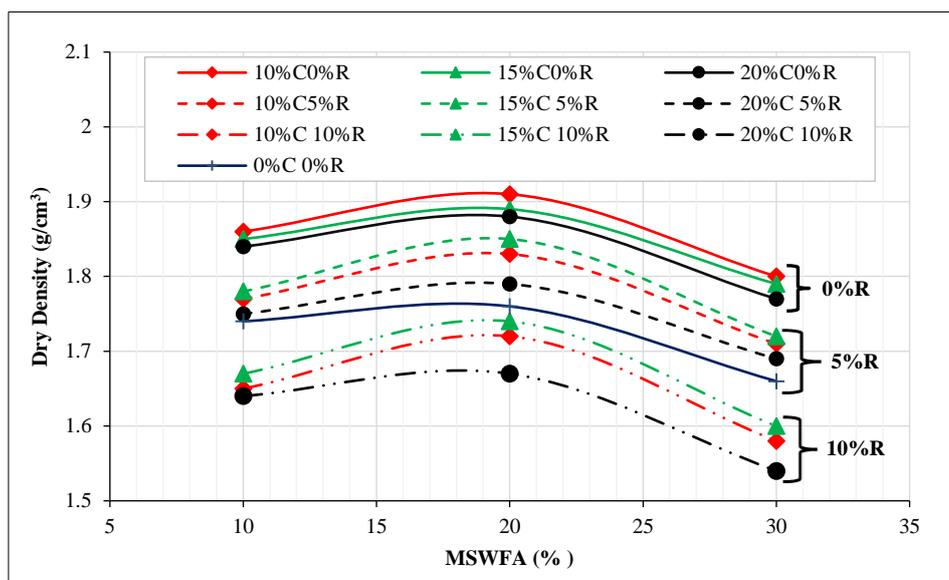
Figure 14. Effect of varying % of Cement, ash, and Rubber on the MDD of soil
