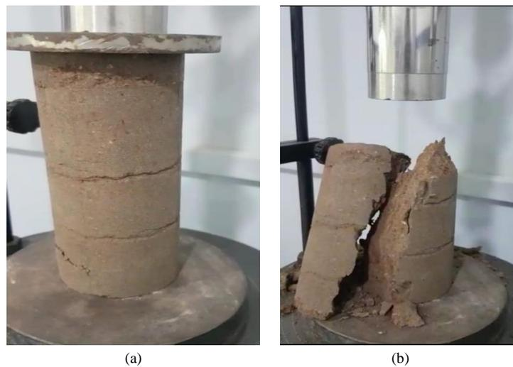
Figure 13. Failure mode of soil cement MSWIFA mix a) just before failure, b) after failure
