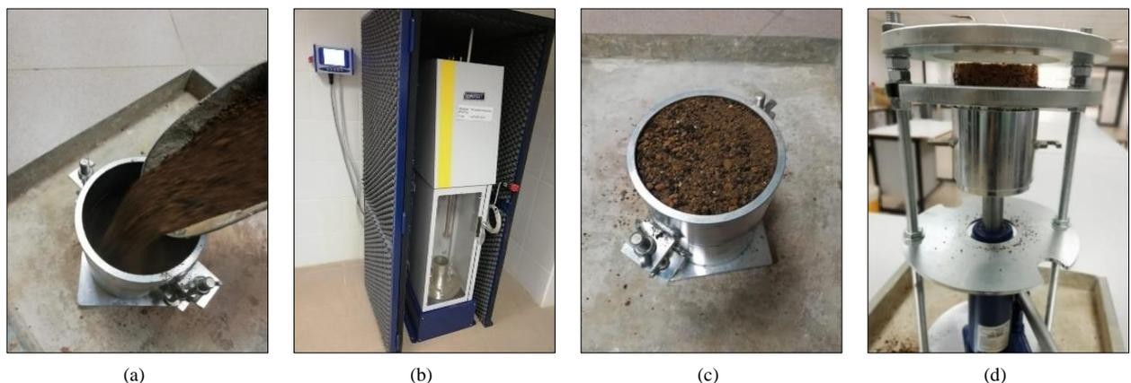
Figure 5. Proctor test a) Mold b) Hammer c) Compacted Soil d) Extruding the Mold
