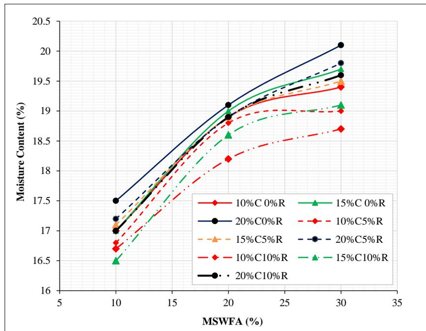
Figure 15. Effect of varying % of Cement, ash, and Rubber on the OMC of soil
