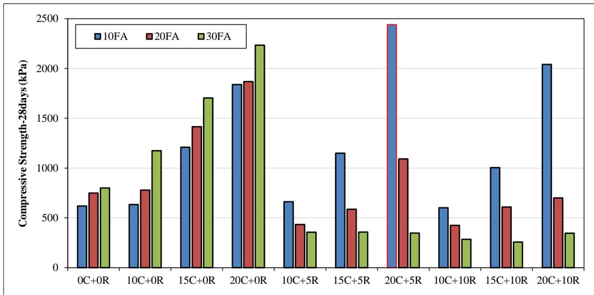
**Figure 17. Compressive strength (28 days) of the mix compared to MSWIFA content for various Cement and Rubber percentages**
