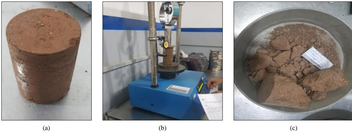
Figure 7. a) Specimen b) Sample at the beginning of UCS test c) Sample after the UCS test
