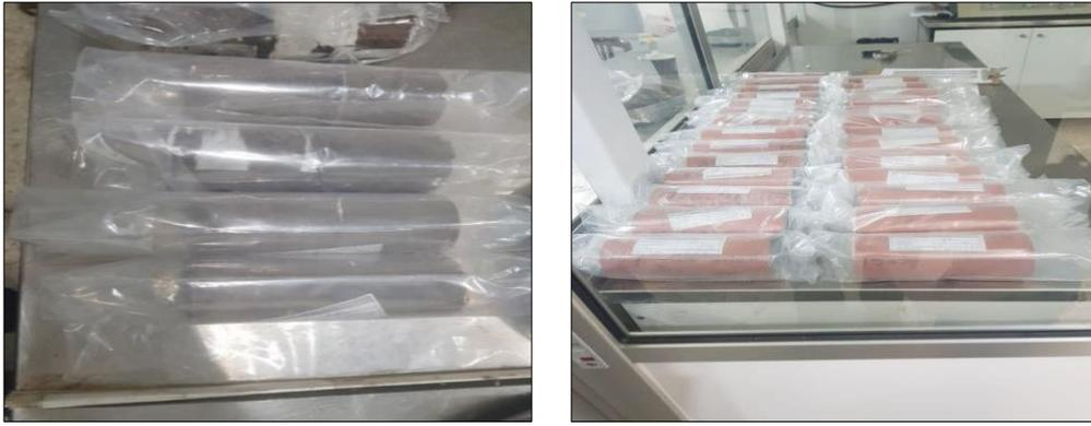
Figure 6. Specimens in room temperature covered in plastic bags
