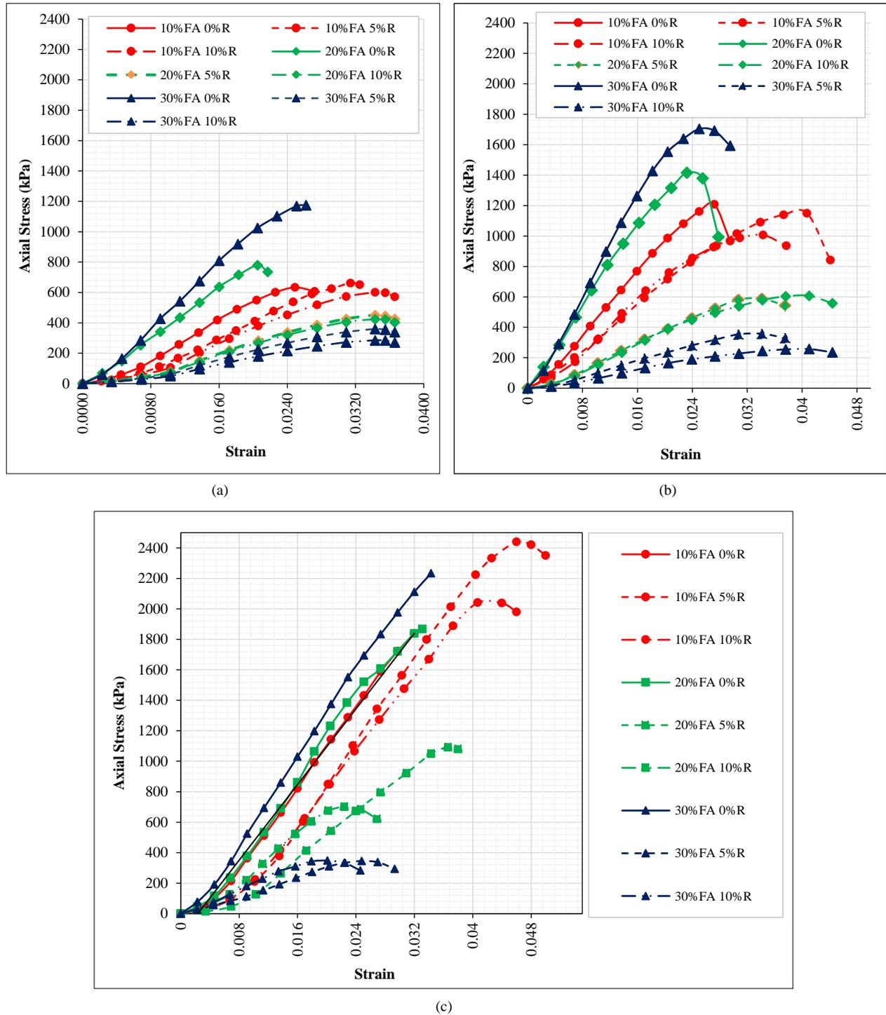
Figure 16. Stress-strain behavior for MSWIFA treated Soil with and without Rubber for varying Cement Contents of (a) 10%, (b) 15%, and (c) 20%
