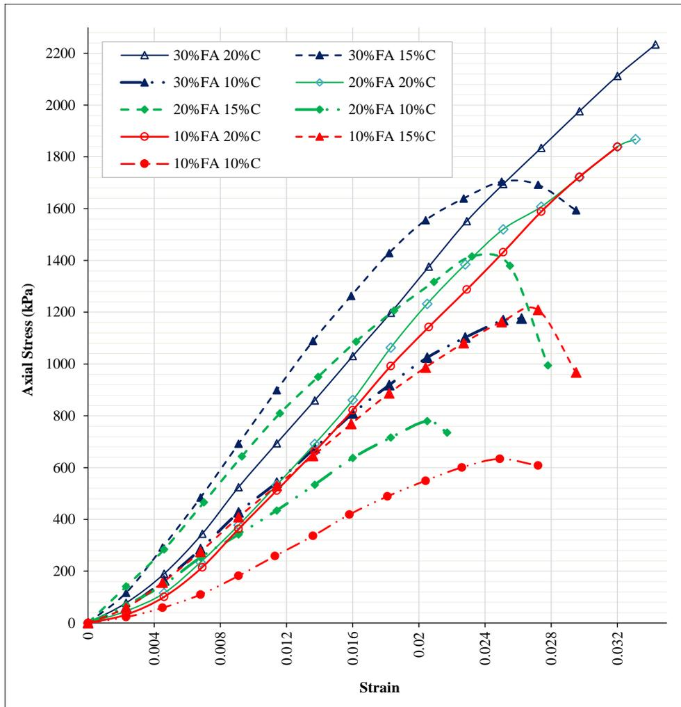
Figure 11. Stress-Strain behavior for Soil mixed with different percentages of MSWIFA and Cement contents at 28 days
