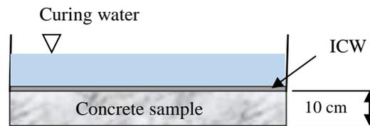
Figure 3. Curing conditions to create ICW
