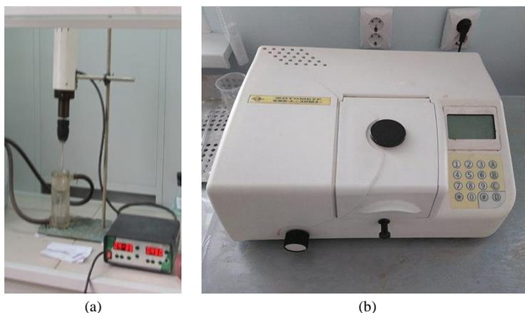
Figure 3. A mechanical mixer BP 8000 EKROS with a thermostatic glass cup (a) and a photoelectric photometer KFK-3-“ZOMS” (b)
