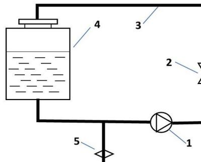
Figure 2. Laboratory installation (1- pump; 2-flow injector; 3- pipeline; 4- container with a solution for processing; 5- drain valve)
