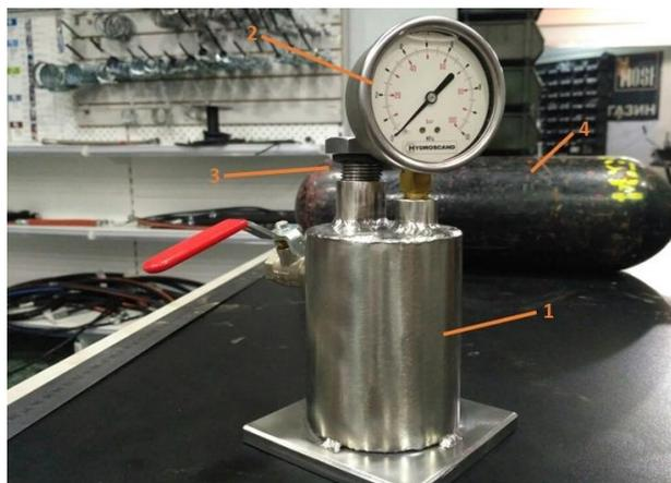
**Figure 7. Installation for studying the effect of pressure on the change in the copper content in the solution**
