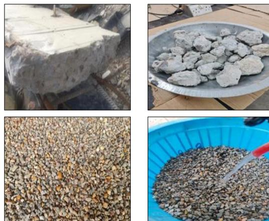
Figure 4. Waste Concrete and RCA particles
