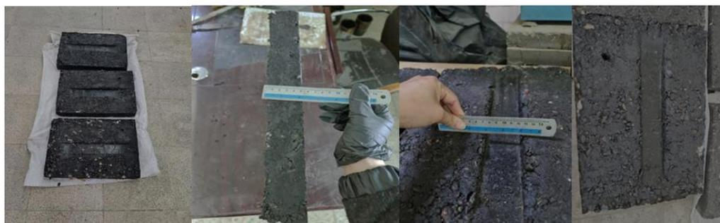
Figure 9. Some of the wheel-tracking specimens
