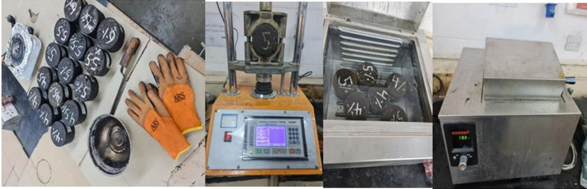
Figure 6. Marshall specimens and test runs
