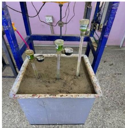
Figure 6. Tensiometer insertion
