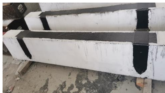
Figure 7. Finished Specimen: AB-U Specimen (view from beam bottom)
