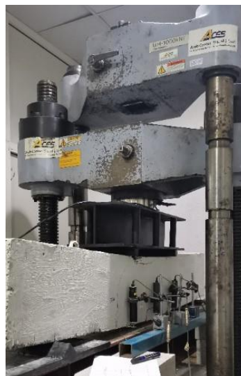
Figure 9. Test setup with beam specimen for flexural loading
